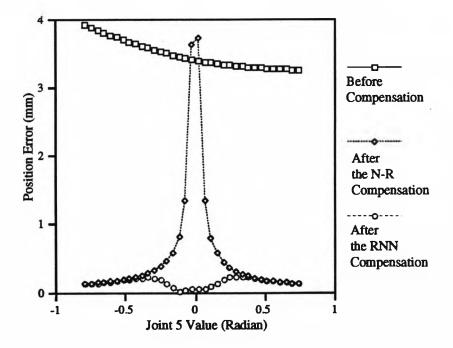
Figure 7.8 Position Compensation Near Robot Singularity
