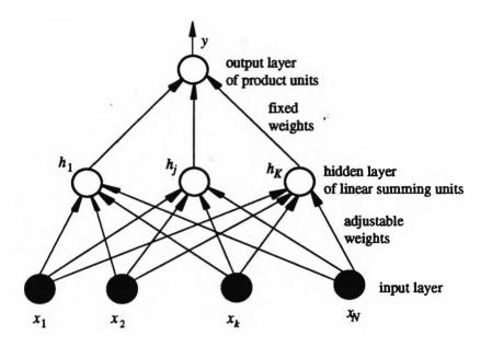
Figure 6.2. A Pi-sigma network with one output (Ghosh and Shin, 1992)
