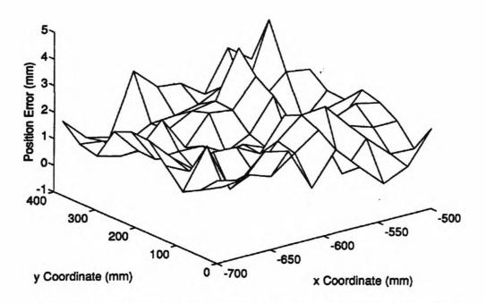
(a). z-axis Constraint Plane Perceived by the Robot Before Calibration
