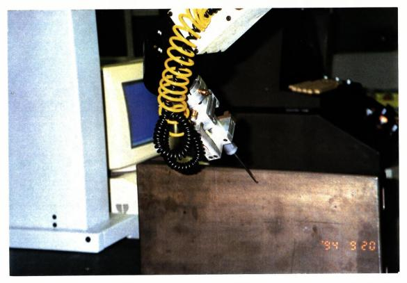
Fig. 5.5 (b). The robot touch an aligned (y-axis ) constraint plane using a probe Figure 5.5. Experimental Set-up for Data Collection
