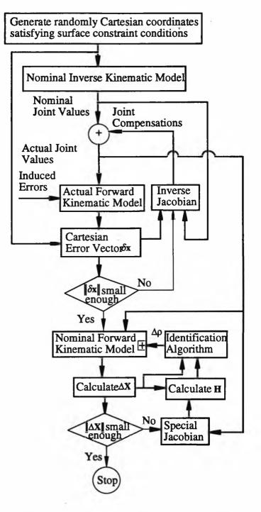
**Figure 5.3. Simulation Program Flowchart**
