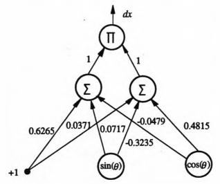
Figure 6.4. NN Representation of Generic Accuracy Model for a One DoF Robot
