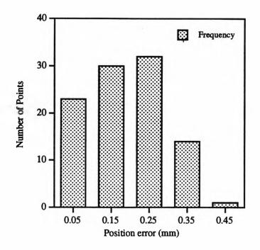
Figure 4.9. The Residual Position Errors Distribution for the 100 Test Points
