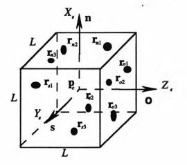
Figure 4.6. The end-effector (measuring cube) co-ordinate system
