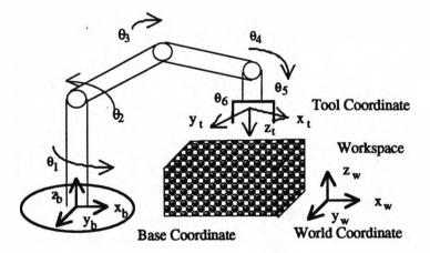
Figure 1.1 Positioning Control of a Robot Manipulator
