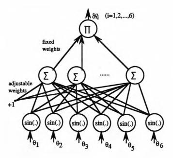
Figure 7.3. Neural Network Architecture for Accuracy Compensation
