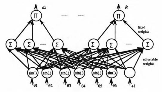
Figure 6.6. Neural Network Architecture for Accuracy Modelling
