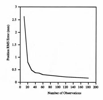
Figure 4.10. The Relationship Between the Observations and Final RMS Errors
