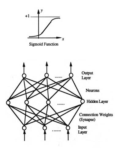
Figure 2.1 Biologically-Inspired Neurocomputing Model --- Multiple-Layered Perceptron with One Hidden Layer
