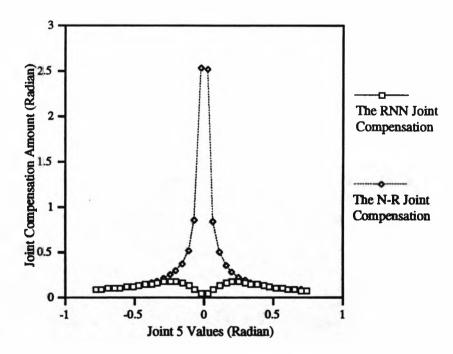
Figure 7.10 Joint Compensation Amount Near Singularity
