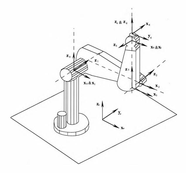
Figure 4.7. Puma Co-ordinate Frame Assignment
