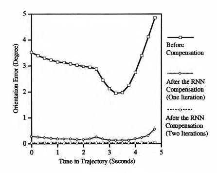
(b). Orientation Error Along the Path Figure 7.6. Accuracy Compensation Along the Path
