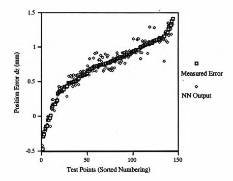
Fig. 6.8 (c) dz Generalisation Test Figure 6.8. NN Generalisation Test for Position Compensation
