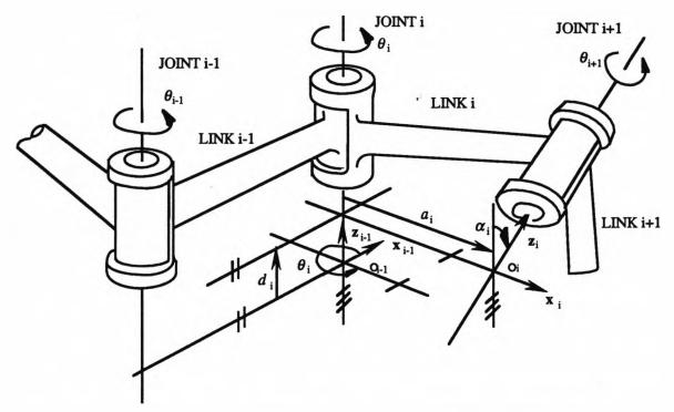
Figure 3.1. Denavit-Hartenberg Parameters for a Revolute Joint
