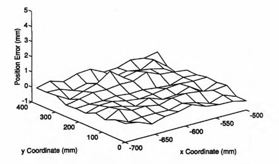
(b) z-axis Constraint Plane Perceived by the Robot After Calibration
