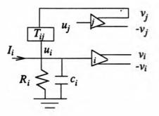
Figure 4.1. Hopfield Neuron Circuit
