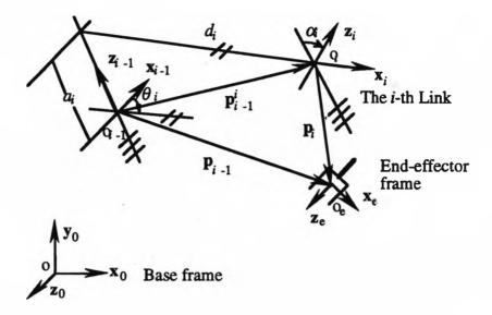
Figure 3.3. Relationship between the differential change of the end-effector frame and the differential changes in the *i*-th link parameters.
