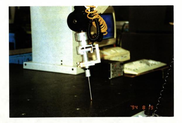
Fig.5.5 (a). Robot touch worktable surface (z-aixs constraint plane) using a probe
