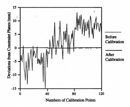
Figure 5.4. Simulation Result with Induced Errors
