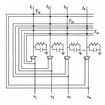
Figure 4.2. Hopfield analogue neural circuit model (Hopfield and Tank, 1986). Black square at intersections represent resistive (weight) connections (with conductance  $T_{ij}$ ).
