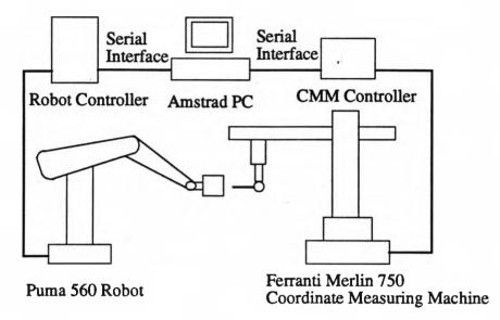
Figure 4.5. Schematic of measurement set-up
