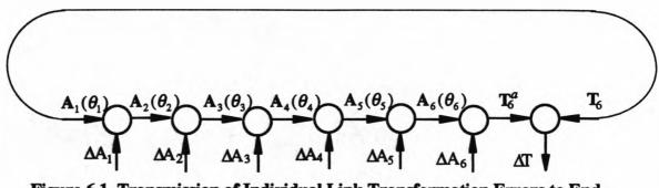
Figure 6.1. Transmission of Individual Link Transformation Errors to End-Effector Error
