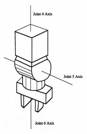
Figure 7.7 Robot End-effector and Wrist Singularity
