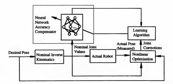
Figure 7.2. a). Training of Neural Network Accuracy Compensator
