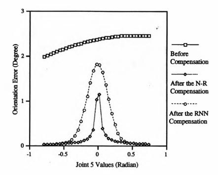
Figure 7.9. Orientation Compensation Near Robot Singularity
