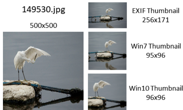
Figure 4: A comparison of 49530.jpg from the Flickr dataset with its embedded EXIF thumbnail, Windows 7 thumbnail, and Windows 10 thumbnail. Image dimensions provided. Windows 7 uses embedded EXIF thumbnails to generate the 96-pixel thumbcache entries, which are not necessarily updated when an image is cropped or otherwise modified.
