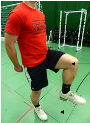
Figure 3.0 represents the orientation of the force plate relative to the location of the participant and the active limb impacting the force plate during a SaE foot-drill manoeuvre.
