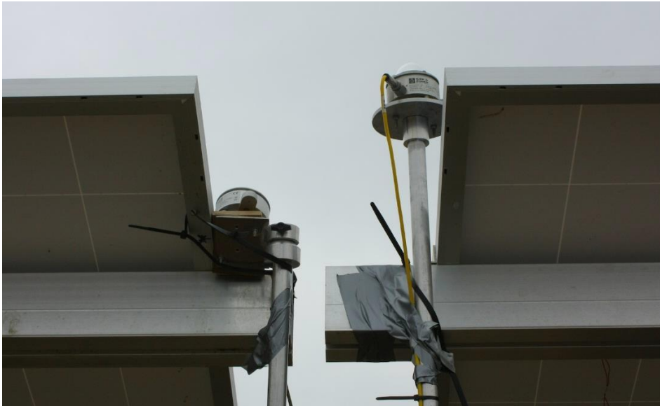
Figure 40 Detail of Horizontal and Upper Slope Pyranometers (p1 & p2)
