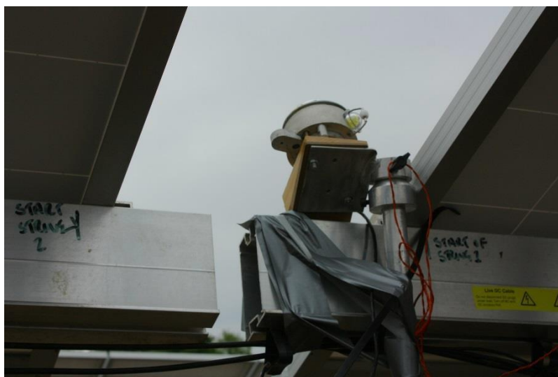
Figure 40 Detail of Horizontal and Upper Slope Pyranometers (p1 & p2)
