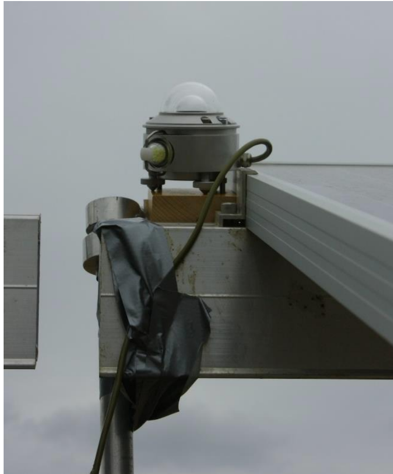
Figure 42 Alignment of Upper Slope Pyranometer (without cover)
