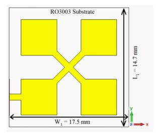
Figure 1. The proposed microstrip antenna array.
