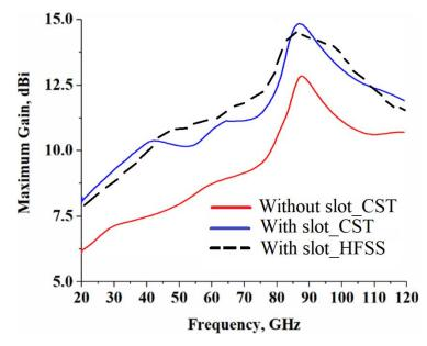
**Figure 4.** Gain response for both cases "with no" slot and "with" slot using two different commercially available 3D full wave electromagnetics simulation tools (CST Microwave Studio® and HFSS<sup>TM</sup>).
