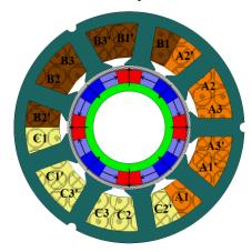
Fig. 4. Cross-section of the 9 slots / 8 poles PMSM.
