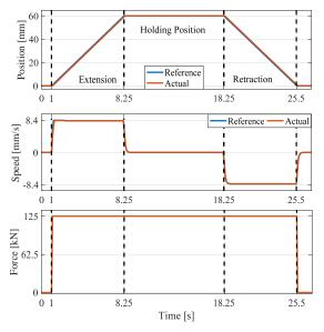
Fig. 25. EMA active-active mode: position (top sub-plot), speed (middle sub-plot), and load force (bottom sub-plot) of the end-rod.
