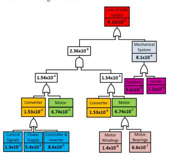
Fig. 3. Fault tree of the considered EMA.
