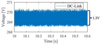
Fig. 21. DC-Link voltage in active-standby operating mode.
