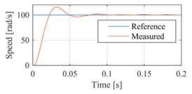
Fig. 22. Measured output speed providing a step reference of 100 rad/s (at no-load).
