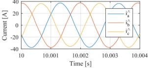
Fig. 20. Measured phase currents in active-standby operating mode.
