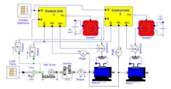
Fig. 24. EMA model in Dymola environment.
