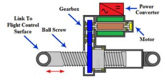
Fig. 1. Example of linear geared EMA.
