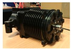
Fig. 5. Assembled PMSM prototype.
