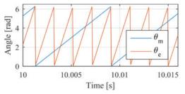
Fig. 18. Measured mechanical and electrical rotor position at 8000 rpm.
