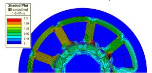
Fig. 8. Flux density map and flux lines distribution at 37.5 A and 8000 rpm.
