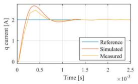
Fig. 16. Output q-current comparison at locked rotor.
