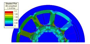
Fig. 6. No-load flux density map and flux lines distribution at 8000 rpm.
