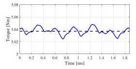
Fig. 9. Instantaneous torque at 37.5 Apk and 8000 rpm.
