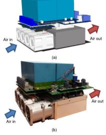
Fig. 12. View of the PEC: (a) Altium 3D and (b) prototype.
