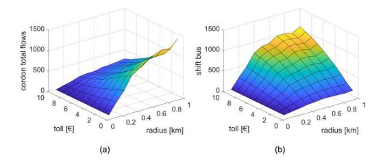
Figure 2. (a) Total car flows passing through the cordon while varying the size of the charged area and the amount of the toll; (b) Number of users that switch transport mode (from car to bus) after the implementation of a pricing strategy on the network.
