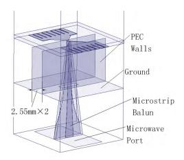
FIGURE 23. Two PEC Walls located symmetrically on the 2 sides of the Microstrip Balun. D-Plane View.
