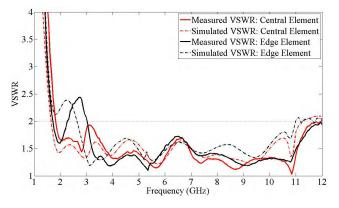
FIGURE 18. Measured and simulated VSWR of the central element and edge element in 1 × 8 phased array.
