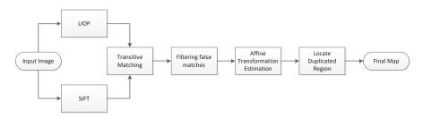
Fig. 1 The framework of the copy-move forgery detection scheme.
