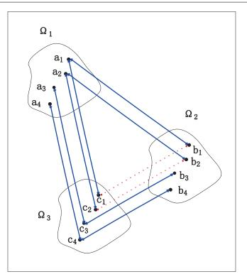
**Fig. 3** The transitive matching. There are three duplicated regions, such as  $\Omega_1$ ,  $\Omega_2$  and  $\Omega_3$ . The initial matching are connected by a solid line, for instance,  $(a_1, b_1)$  and  $(a_1, c_1)$ . The transitive matching are connected by a dotted line, for instance,  $(b_1, c_1)$ .
