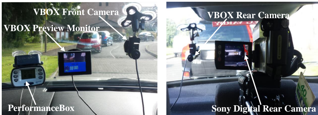
d: The Front (LEFT) and Rear (RIGHT) view setup of instrumentation in the Test Vehicle
