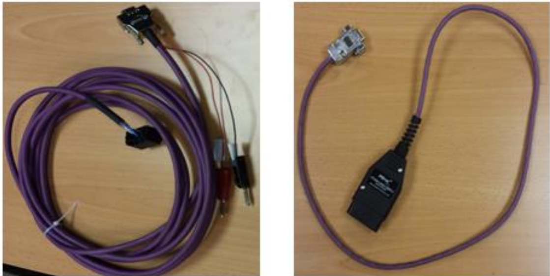
Figure 3-3: The 5-metre power supply high-speed Radar Sensor - CAN-Bus cable (left) and CAN-OBD-II diagnostic 1-metre cable (right)
