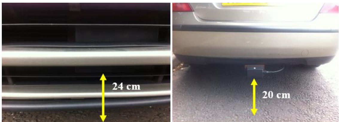
Figure A3-17: The mounted heights of the radar sensors on the instrumented vehicle (Left: Front and Right: Rear)
