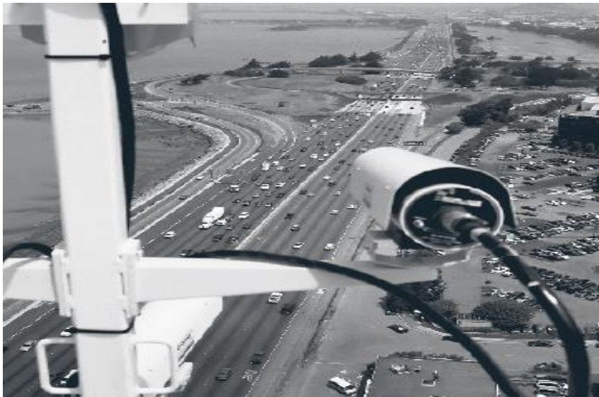
Figure 2-1: Typical digital video camera mounted on top of a building overlooking the highway to record vehicles trajectories data for NGSIM database (Source: Halkias and Colyar, 2006)
