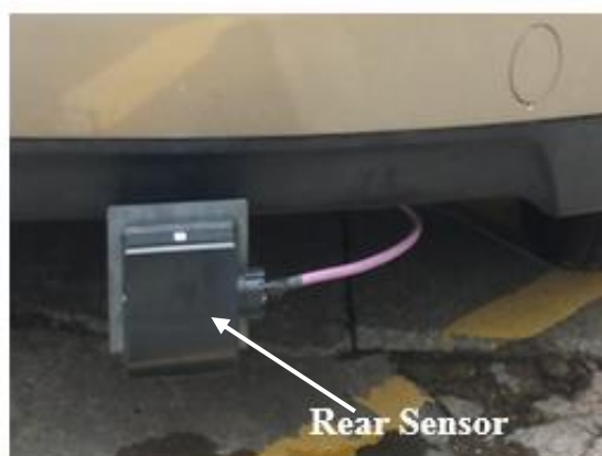
a: ARS 308-2 radar sensors mounted at back (LEFT) and front (RIGHT) of Test Vehicle
