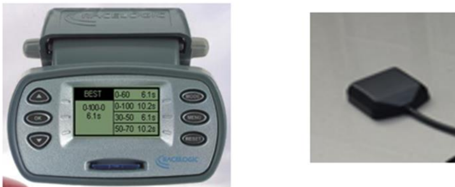
Figure A3-7: PerformanceBox and GPS antenna (right) used for the study (manufactured by Racelogic Ltd)
