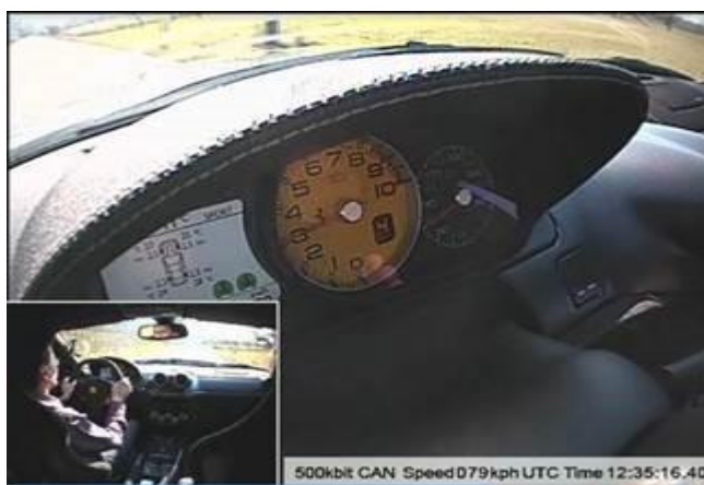
Figure A3-19: Video VBOX Picture in Picture camera view of RPM gauge in car (Source: Racelogic Ltd)
