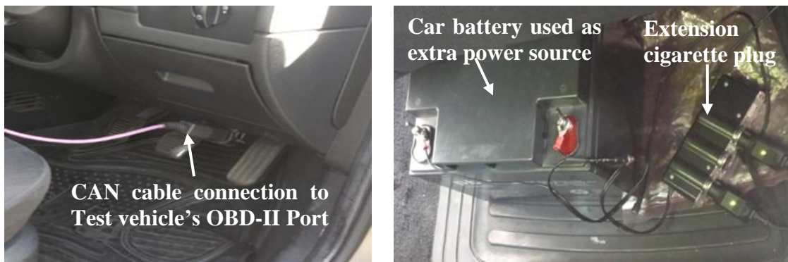
b: The Test Vehicle's OBD-II – CAN-USB connection (LEFT) and Stand-alone car battery supplying power to PB and VB (RIGHT)
