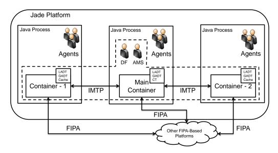
Figure 9: JADE architecture based on [98].
