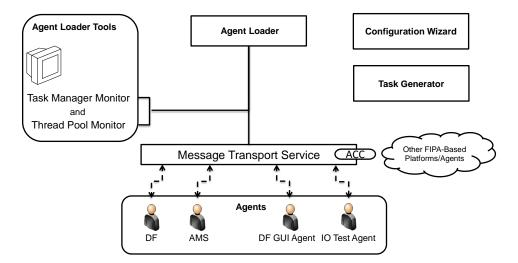
Figure 14: FIPA-OS architecture based on [113].
