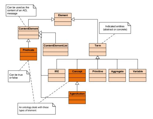
Figure 10: The content reference model (based on [109]).
