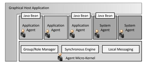
Figure 13: MadKit architecture (based on [112]).
