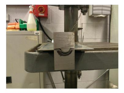
Figure 128 Forming door for cable exit
