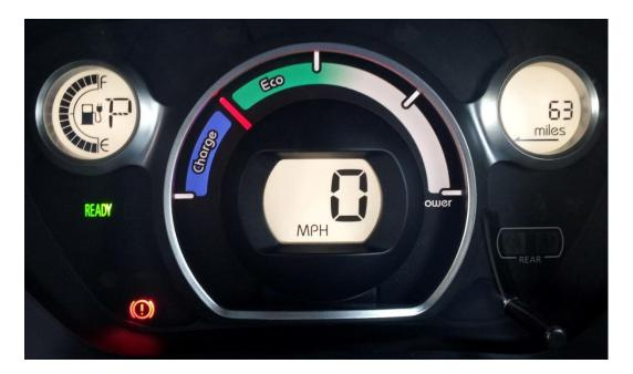
Figure 84 In-car display – suggested distance the vehicle can travel shown on right hand side instrument.
