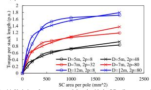
Fig. 14. Variation of torque per stack length with the SC coil area per pole of generators with a range of stator outer diameter and pole number. Base values:  $5\text{MNm}(D=5\text{m}\ 2p=8)$ ,  $7\text{MNm}(D=5\text{m}\ 2p=48)$ ,  $15\text{MNm}(D=7\text{m}\ 2p=32)$ ,  $9\text{MNm}(D=7\text{m}\ 2p=80)$ ,  $5\text{MNm}(D=12\text{m}\ 2p=8)$ ,  $30\text{MNm}(D=12\text{m}\ 2p=80)$ .
