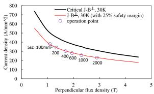
Fig. 13. Critical current density - flux density characteristics of the SC material. The operating current density and maximum self-induced  $B_{\perp}$  in the SC coil for designs with a range of SC coil area per pole are shown as operation points. D=7m, 2p=32.
