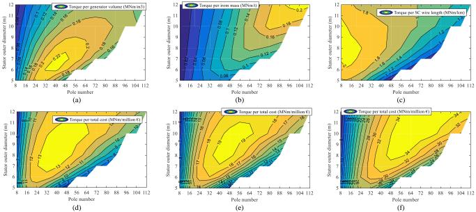
Fig. 12. Contours of (a) torque per generator volume, (b) torque per iron mass, (c) torque per SC wire length, (d) torque per total cost, SC=100e/m, (e) torque per total cost, SC=60e/m, (f) torque per total cost, SC=20e/m.
