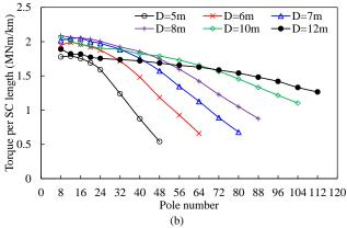
Fig. 7. Variation of length ratios of SC wire straight length to total length and torque per SC length with pole number for different stator outer diameters, torque=10.5MNm. (a)  $L_{sc(stack)}/L_{sc(total)}$ . (b) Torque per SC total length.
