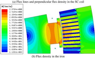
Fig. 10 No load flux lines and flux density distribution, D=7m, 2p=32, (a) flux lines and perpendicular flux density in the SC coil, (b) flux density in the iron.
