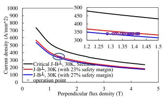
Fig. 11. Critical engineering current density - flux density characteristics of the SC material. The operational current density and maximum self-induced  $B_{\perp}$  in the SC coil for designs in TABLE III are also shown as operation points.
