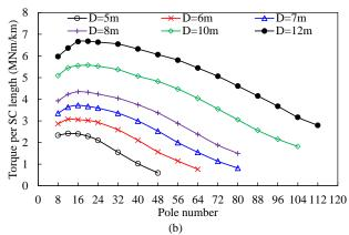
Fig. 6. Variation of SC wire length and torque per SC length with pole number for different stator outer diameters, the end length of SC coil is not considered.
