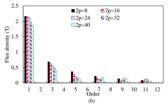
Fig. 3. No load flux density in the middle of airgap, D=5m, (a) Waveforms. (b) Spectra
