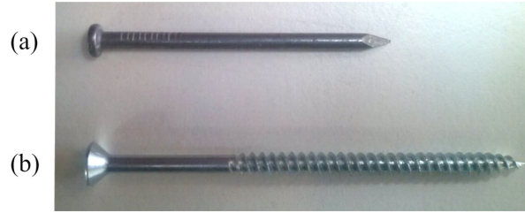
Figure 7: (a) Bright smooth wire nail 3.0 mm diameter \times 52 mm long, for the stud-to-beam connections. (b) Screw for the stud-to-beam connections: 3.2 mm diameter (smooth shank) \times 75 mm long.
