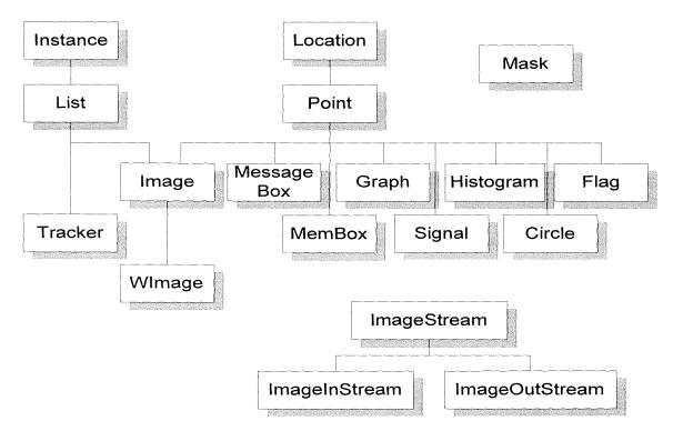
**Figure 14:** Class hierarchy of the Multi-resolution Image Sequence Analysis (MISA) software. Base classes are shown at the top with those inheriting their characteristics linked from below.
