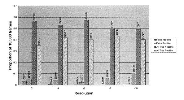
**Figure 48:** Binary detection performance of the algorithm as a function of operating resolution on analysis of sequence  $BC5_1$ . The algorithm's output is classified according to whether it is correct (True/False) and whether there are pedestrians present (Positive/Negative). Resolution is expressed as a fraction of 256 pixels (e.g. r4 = 256/4).
