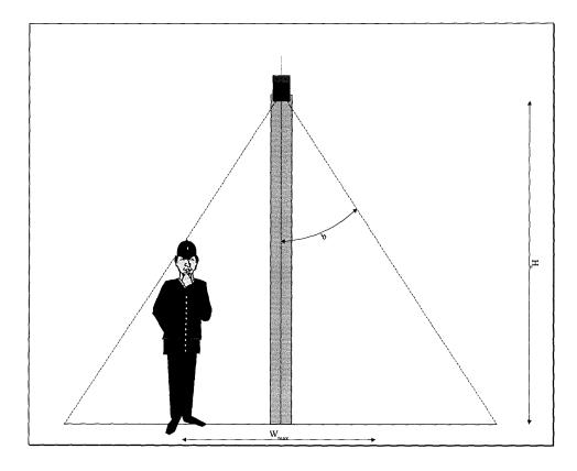
**Figure 16:** View parallel to the roadside showing how constraints such as pedestrian height and the camera's field of view and mounting height are linked to the width of detection zone that can be used.
