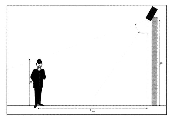
**Figure 15**: Side view indicating how constraints such as pedestrian height and the camera's field of view and mounting height are linked to the length of detection zone that can be used.
