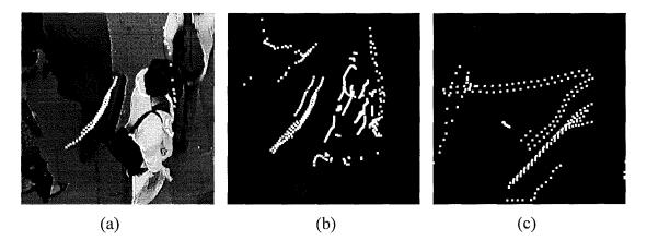
Figure 28 Feature Tracking: Frame (a) shows the history of a number of tracks currently being tracked that have been overlaid onto the latest image. Each white
