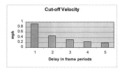
Figure 35: Variation in cut-off velocity for equipment used in this work (p = 0.5,  $H_{cmin} = 3.0m$ ,  $H_{pmax} 2.0m$ ).
