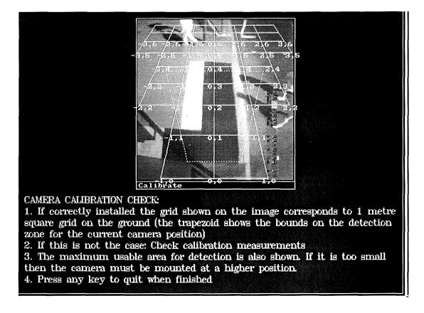
**Figure 4. Typical Check Calibration Screen**
