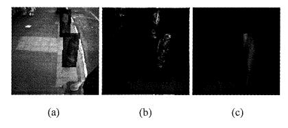
**Figure 41:** The result of the evidence integration process (c) shown with the detected pedestrians in the original image (a) and the match image (b).
