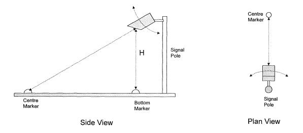
Figure 2. Camera head positioning (mount allows rotation about horizontal (pitch) and vertical (yaw) axes)
