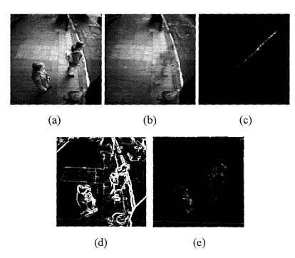
**Figure 33:** Performance of the persistence filter under diffuse lighting conditions. The relationship between the current image (a) and background (b) is indicated in the scattergraph (c). The selection of features of interest from the gradient features in the current image (d) by the matching operation is shown in (e).
