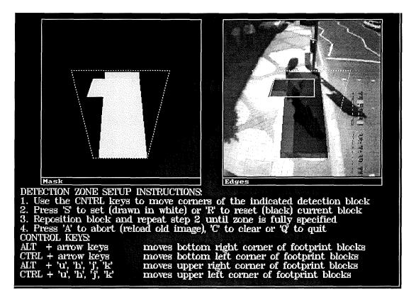
Figure 5. Sample view of Detection Zone specification
