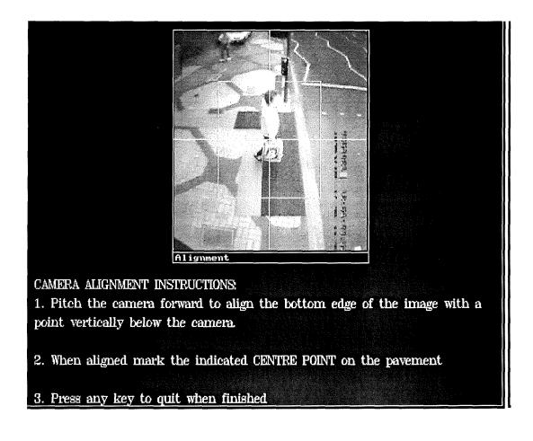
Figure 1. Typical Align/Check Screen
