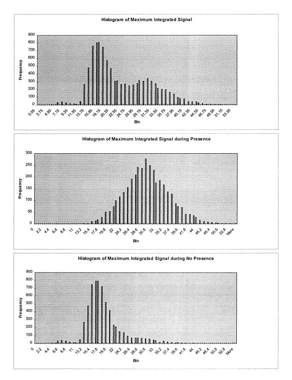
**Figure 45:** Distributions of Maximum Integrated Signal from the Evidence Map monitored over a 10,000 frame test sequence.
