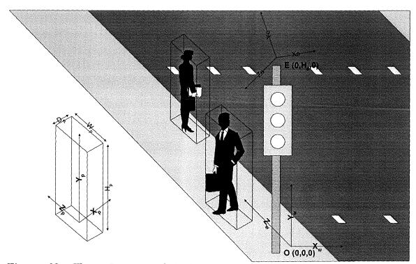
**Figure 38:** Three Dimensional Pedestrian Model. The diagram shows the relationship of the world co-ordinate system (defined with respect to an origin at the base of the signal pole, with the z axis along the surface of the pavement) to the camera co-ordinate system defined from an origin at the camera position with the z axis looking down at the centre of the detection zone. Both world and eye co-ordinate systems are left-handed.
