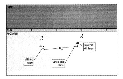
Figure 39: Plan view of detection area showing installation parameters
