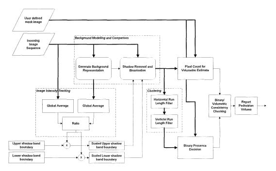
**Figure 29** *Pixel Classification Algorithm. Dark and light paths indicate image and parameter flows respectively.*
