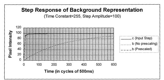
**Figure 32:** The response of the background filter to a step input is shown along with the pre-scaled version used to accelerate the initialisation process.
