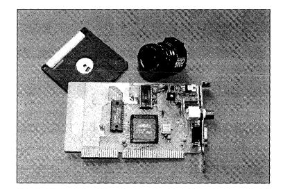
Figure 12: Frame-grabber designed for ASIS image sensors
