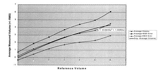
**Figure 49:** Graph of Actual Pedestrian Volume (from reference data) against Average Volume output from the detection algorithms. The upper and lower traces show the RMS deviation of the measured values from the reference.
