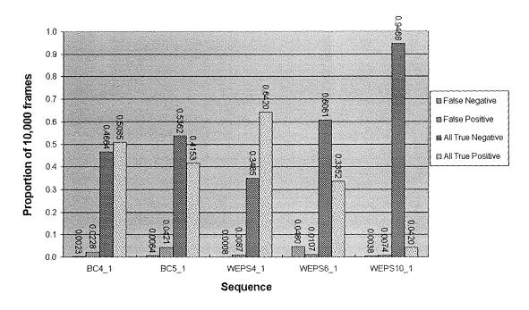
**Figure 47:** Binary detection performance of the algorithm on a frame-by-frame analysis of five test sequences. The algorithm's output is classified according to whether it is correct (True/False) and whether there are pedestrians present (Positive/Negative) as a proportion of the 10,000 frames analysed.
