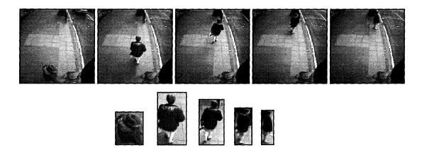
**Figure 17**: The effects of perspective causing a change in scale and viewpoint as a function of pedestrian position in the scene are illustrated by the above sequence. Underneath the pedestrian is shown clipped from each frame to make the effect on scale, viewpoint and image resolution more apparent. Source WEPS4\_1\_3068-88.
