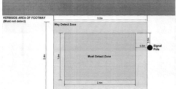
Figure 3: Specified typical detection zone for the Puffin crossing
