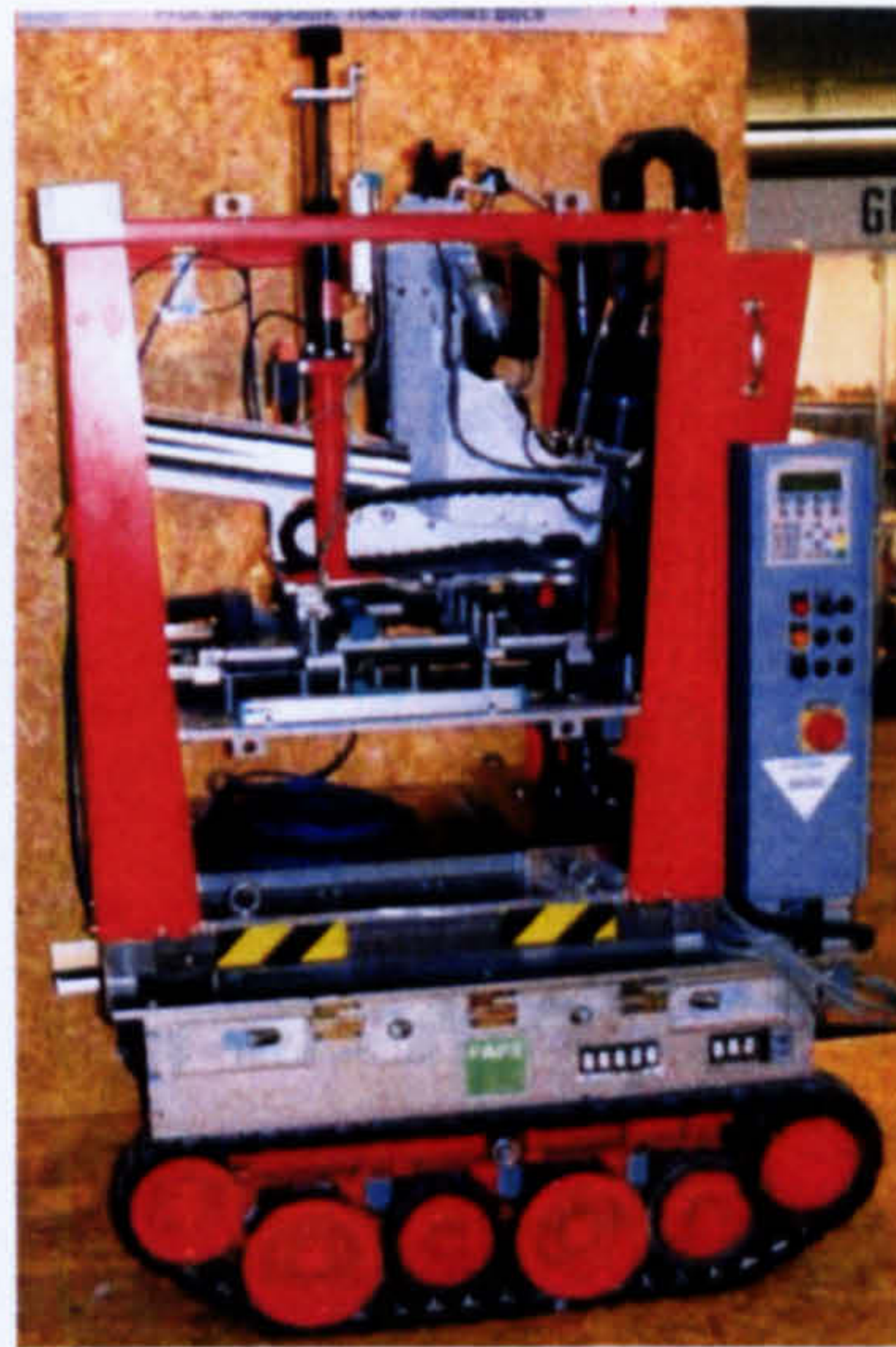
Figure 3.22: Prototype modular construction robot system Courtesy: TU München, Lehrstuhl br+i
