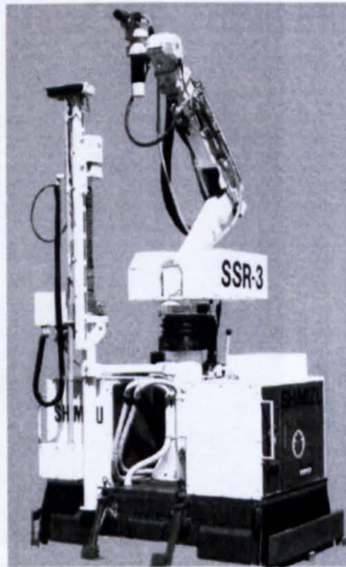
Figure 3.20: SSR-3 steel fireproofing spray application system Courtesy: Shimizu Corporation
