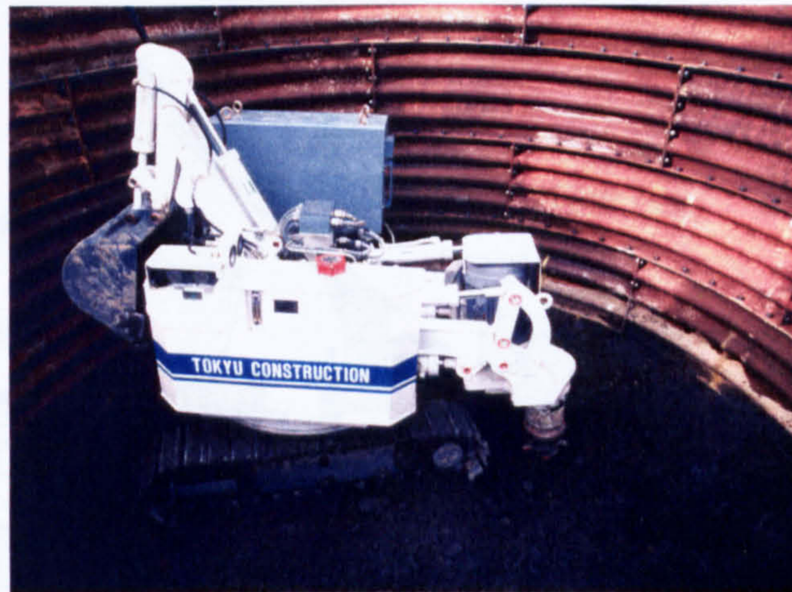
Figure 3.28: Tele-operated excavation system Courtesy: Tokyu Construction Co. Ltd.
