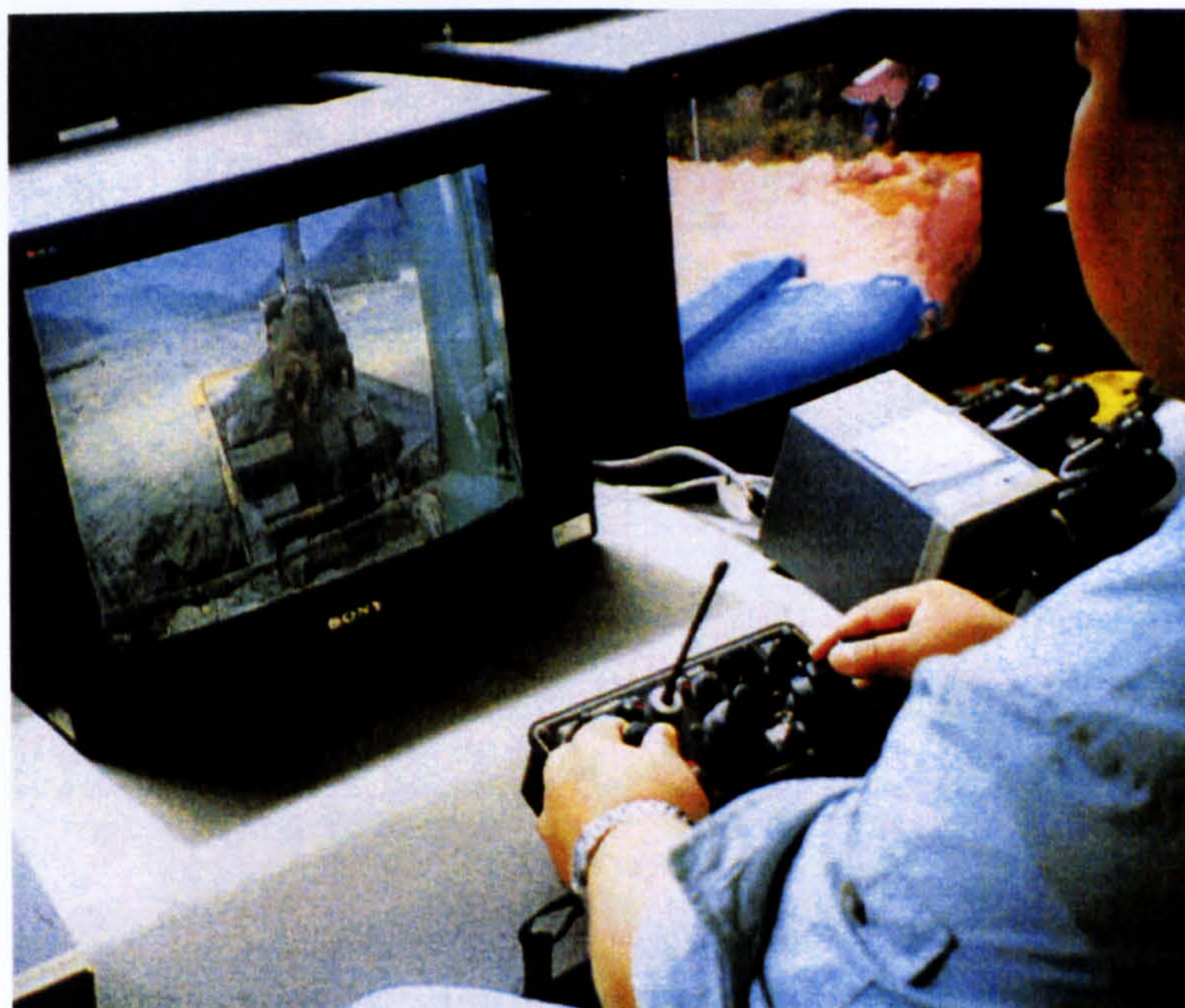
Figure 3.7: Radio controlled tele-operation Courtesy: Kajima Corporation
