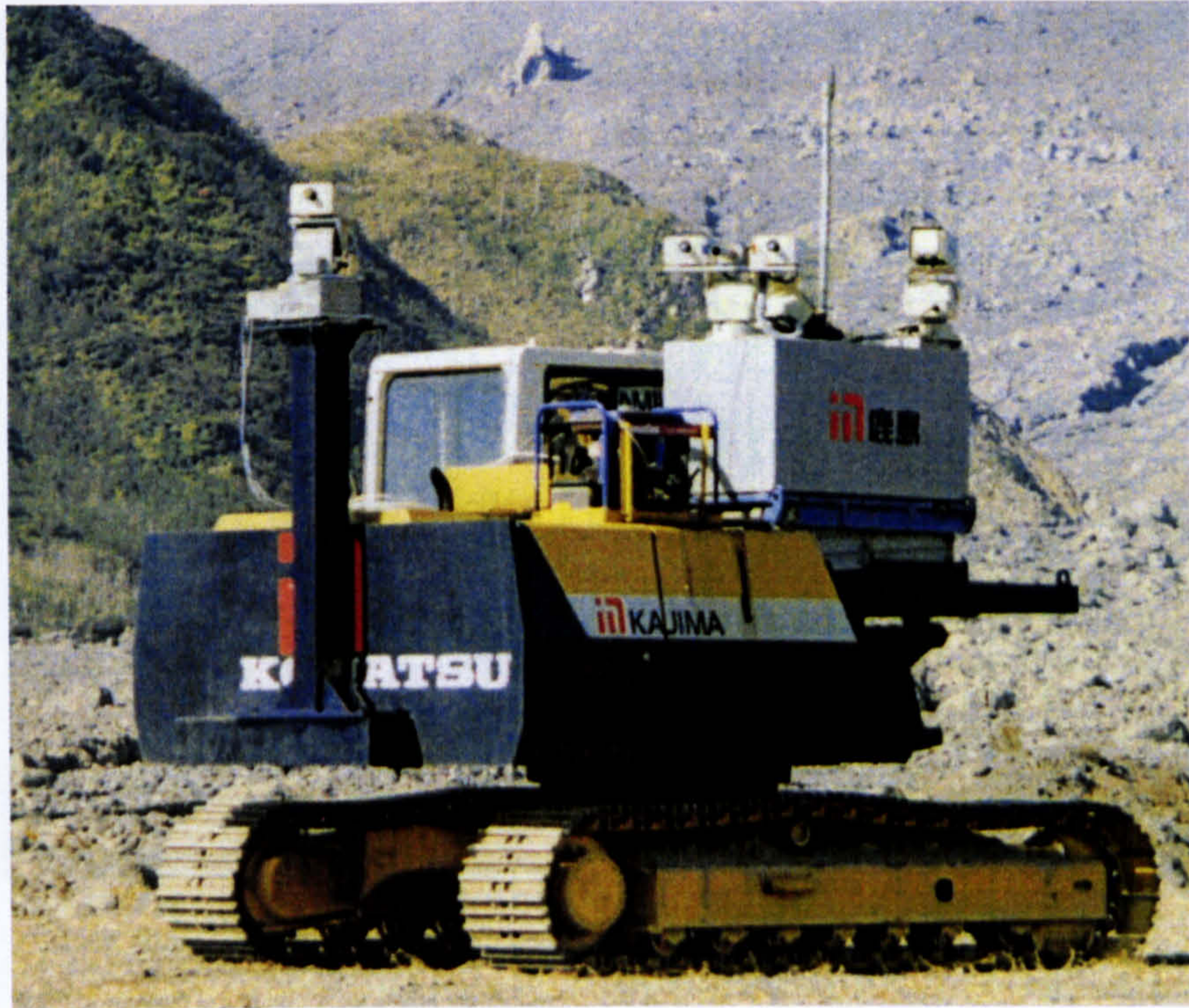
Figure 3.6: Radio controlled excavator Courtesy: Kajima Corporation
