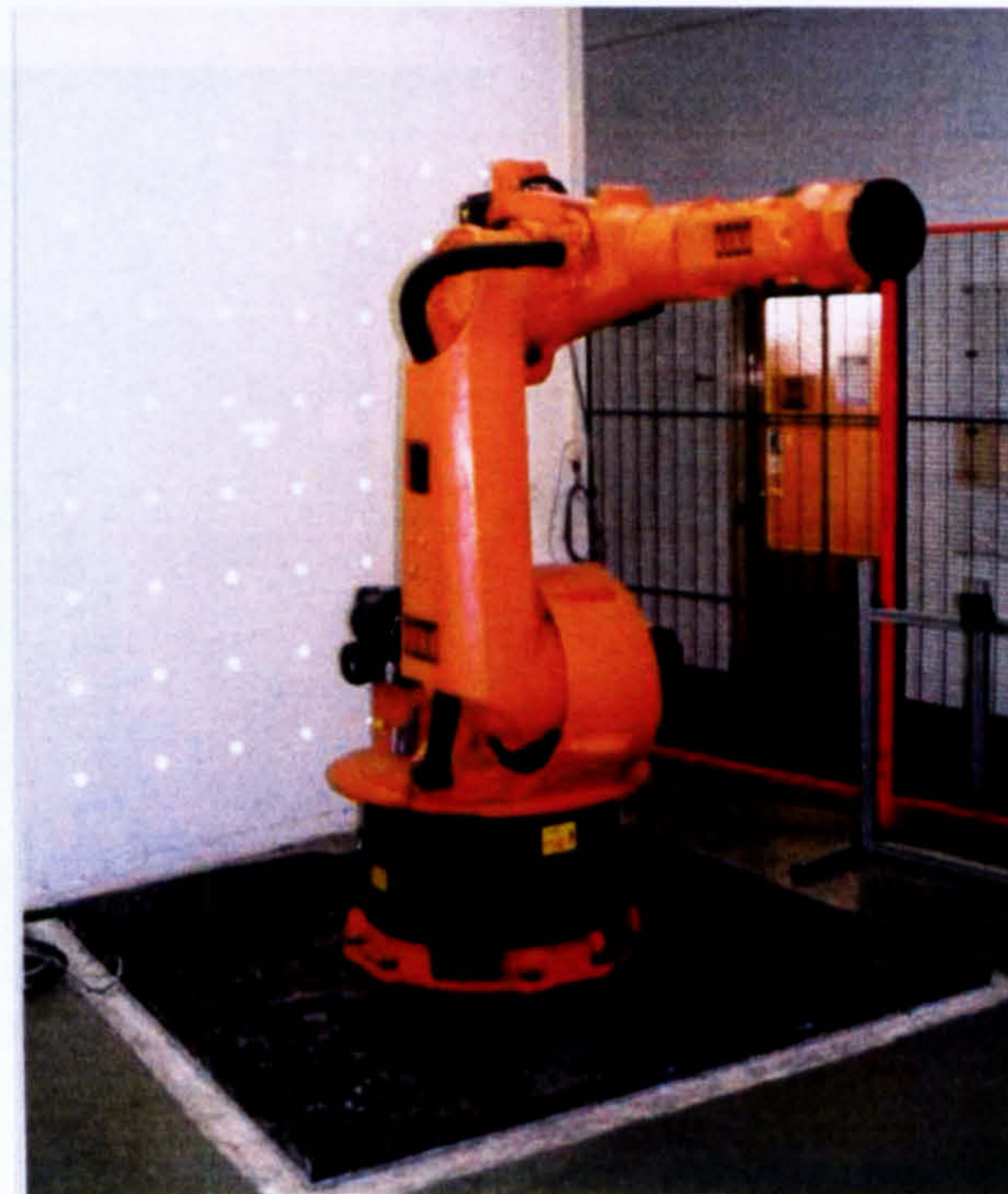
Figure 3.15: Kuka KR210 heavy-duty manufacturing manipulator Courtesy: University of Stuttgart, ISW
