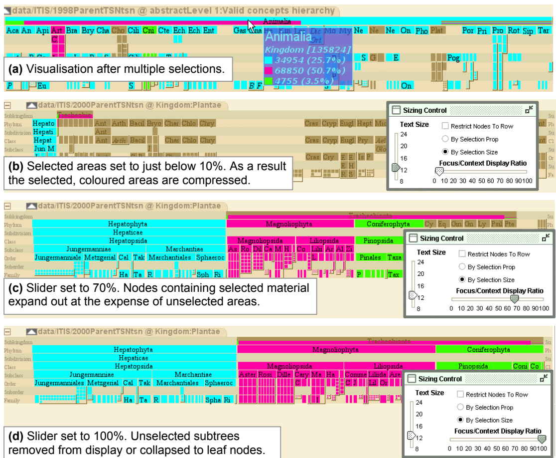
Figure 10. Multiple selections with the Focus & Context slider. (a) shows a standard result of a multiple selection. Changing the ratio of focus to context to extremes can either (b) compress subtrees with selected nodes, (c) give some space to all subtrees, or (d) hide all subtrees that have no selected nodes.
