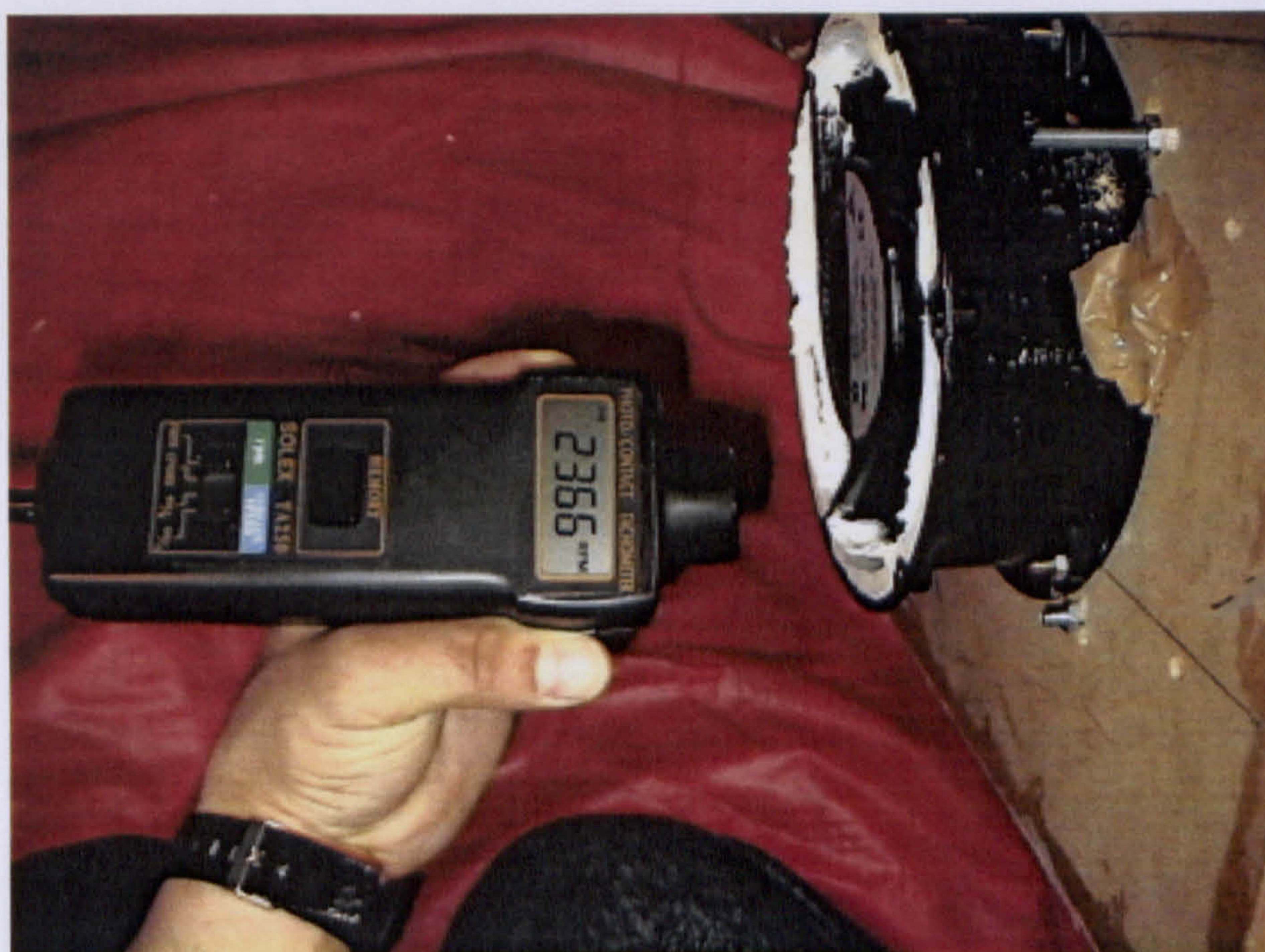
Fig. 3.4: Handheld optical tachometer for measuring fan rotational speed (r/min)
