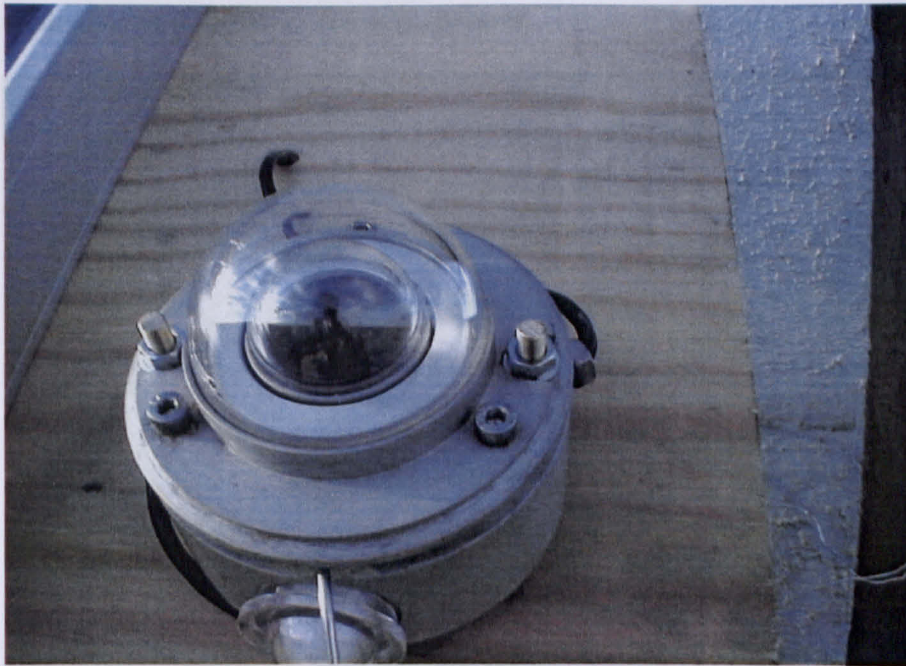
Fig. 3.3: Kipp and Zonen pyranometer used throughout the present research.
