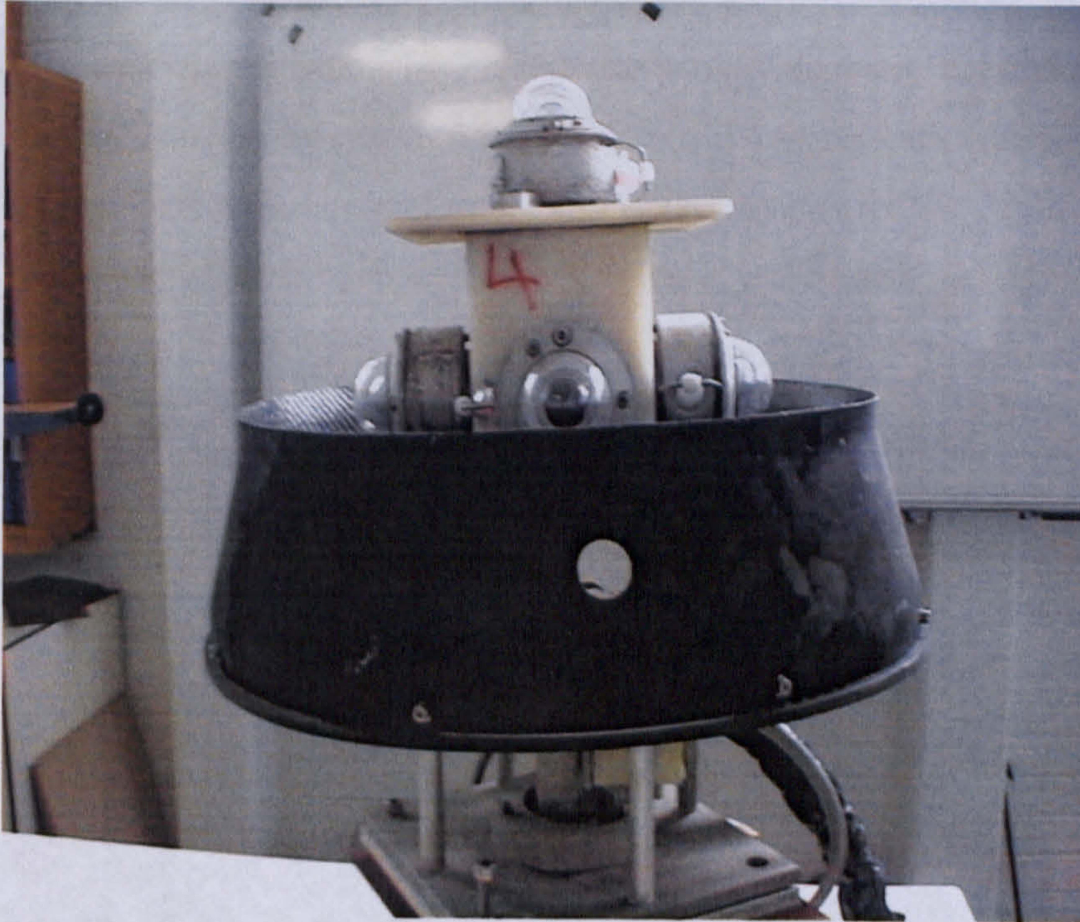
Fig. 5.10: Quintuple pyranometer set for measuring horizontal and vertical global irradiance.
