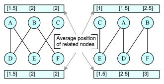
Figure 2. In the left-hand diagram, the node pairs B & C and E & F have the same median and mean values according to the positioning of their immediately connected neighbours. The layout of the nodes will therefore not automatically improve to the layout seen in the right hand side version.
