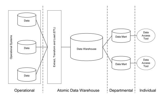
Figure 4. Hub and Spoke Architecture
