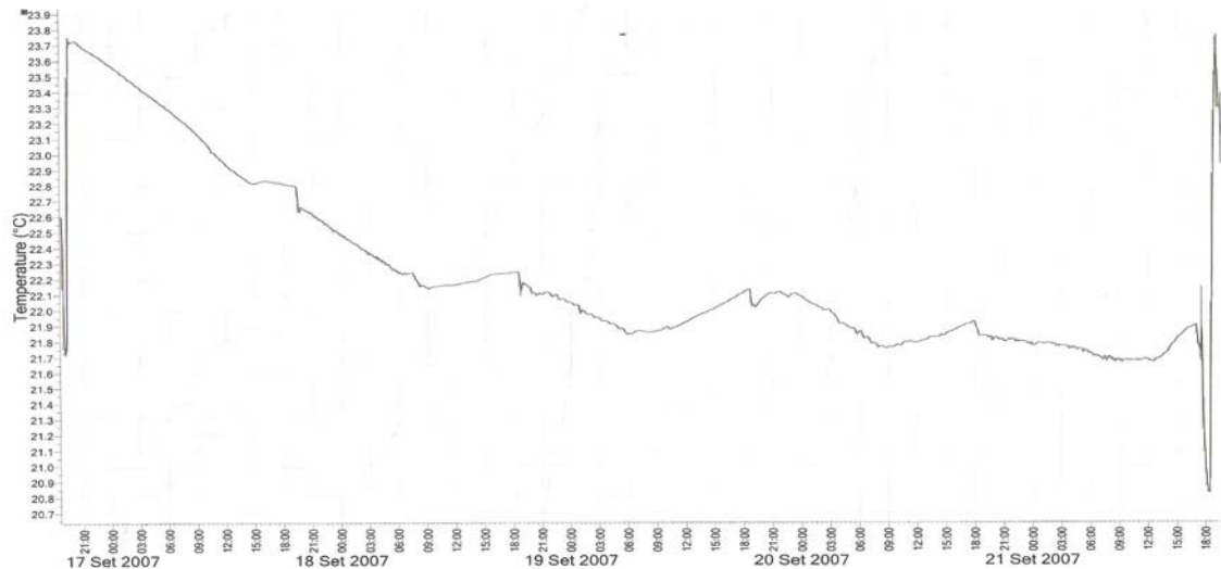
Figure 6.14 – Temperature variation during the third experiment in the tank without light.
