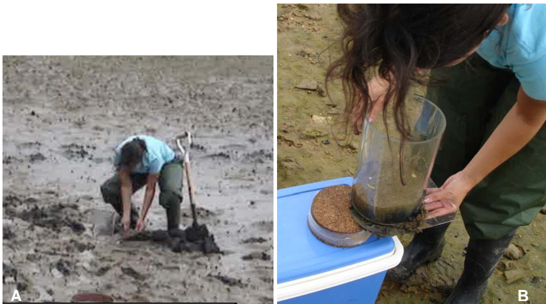
Figures 6.6– A - Sampling the sediment cores. B – Placing the cork stoppers.
