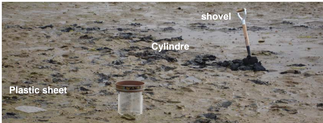
Figure 6.5– Equipment for the sampling.
