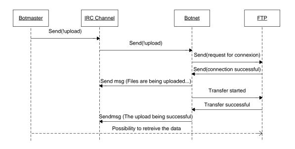
Figure 8 - UML Diagram of FTP module calls
