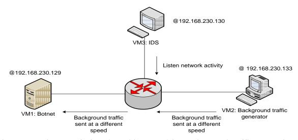
Figure 11 - Diagram of Virtual Machines used for Background traffic generation
