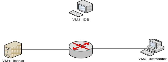
Figure 10 - Diagram of experimental Virtual Network
