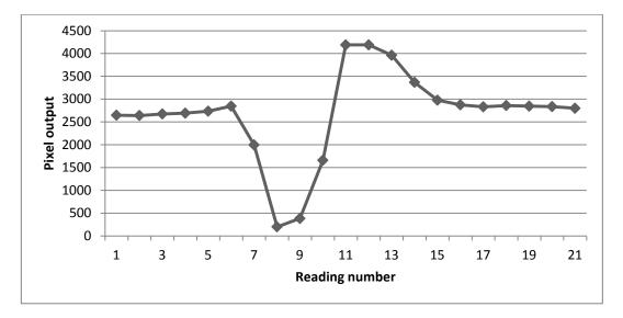
Fig. 3. Output from a single pixel in response to a hand swipe
