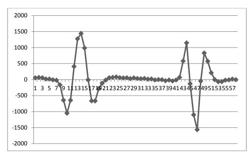
**Fig. 6.** Using the detector in differential mode to detect a hand swipe moving backwards and forwards across the detector.
