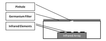
Fig. 2. Optical arrangement.
