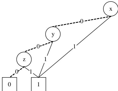
**Figure 6:** Reduced Binary Decision Diagram for the function
