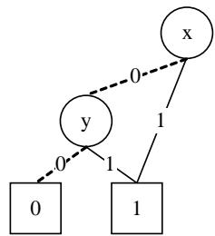
**Figure 5:** Reduced Binary Decision Diagram for the function
