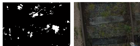
Figure 3. (a) Output mask showing detected vegetation, (b) Original image.
