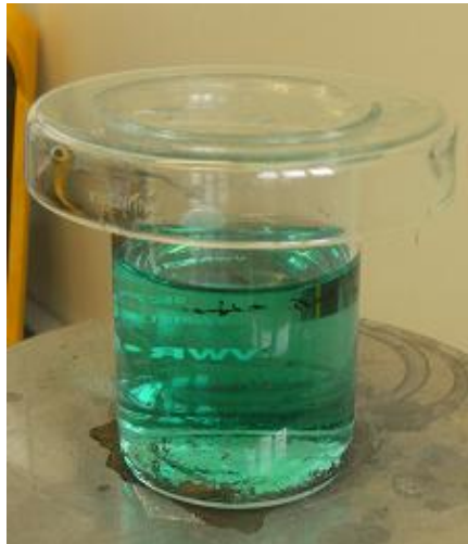
Figure 18. Acidic Slotonip 1850 electroless nickel solution. Green colour synonymous with the presence of green octahedral hexaqua nickel ions [\text{Ni}(\text{H}_2\text{O})_6]^{+2}
