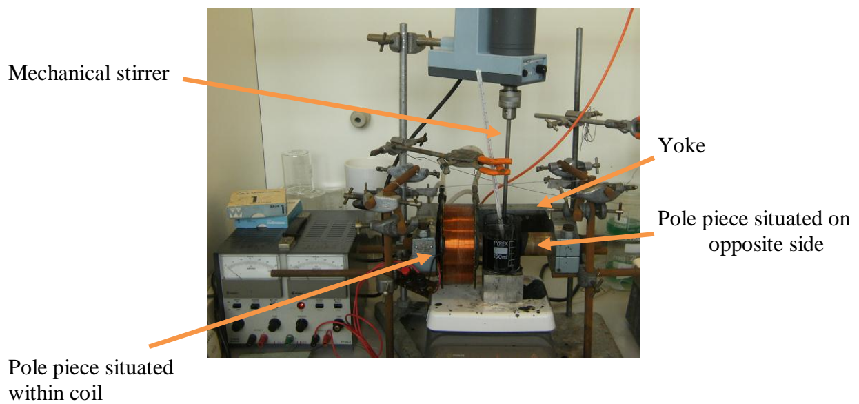
Figure 79. Experimental setup for magnetic Ni – LSM co-deposition process
