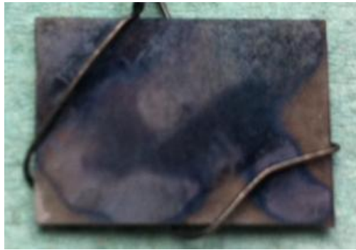
Figure 85. Image of acidic electroless nickel – LSM coating manufactured under 65 mT magnetic field strength at an agitation speed of 300 rpm.
