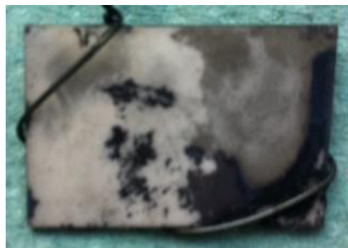
Figure 87. Image of acidic electroless nickel – LSM coating manufactured under 65 mT magnetic field strength at an agitation speed of 500 rpm.
