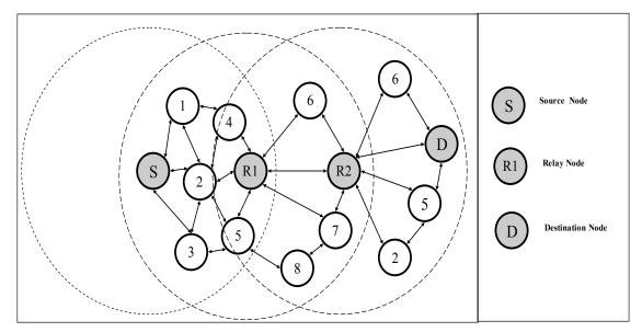
Figure 3-4: Example of PDRD scheme.
