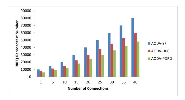
Figure 3-12: RREQ rebroadcast number VS. number of connections for a network of 100 nodes in 1000m x 1000m area.
