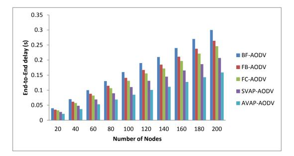
Figure 4-16: Performance of the proposed schemes in terms of end-to-end delay VS number of nodes.
