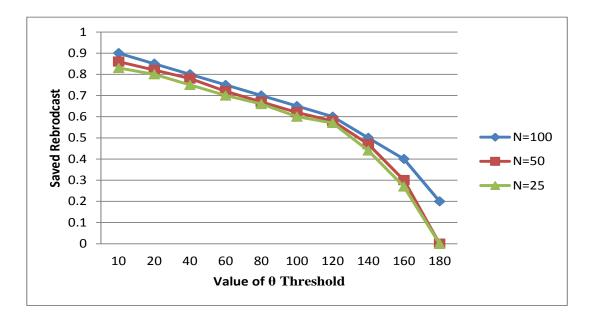
Figure 4-4: RREQ saved rebroadcast vs. Value of  $\theta$  Threshold over different network densities.
