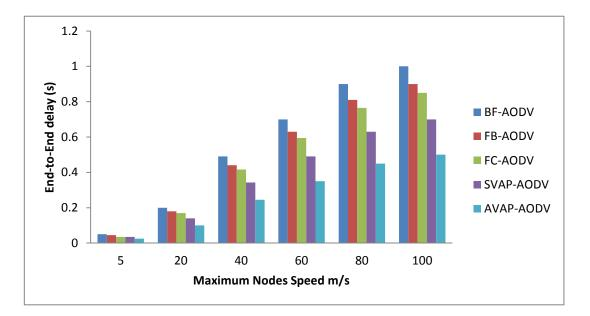
Figure 4-11: Performance of the proposed schemes in terms of end-to-end delay VS nodes speed m/s.
