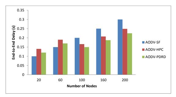
Figure 3-11: shows end-to-end delay vs. number of nodes for all the proposed schemes.
