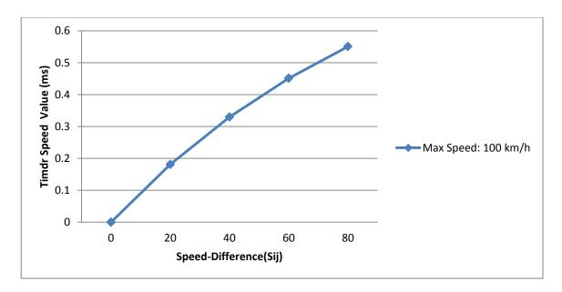
Figure 5-4: Timer speed value for different speed difference values.
