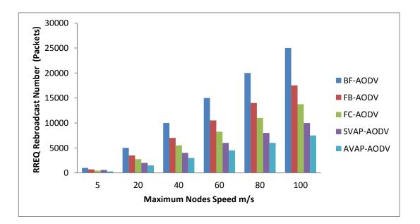
Figure 4-8: Performance of the proposed schemes in terms of RREQ rebroadcast number VS nodes speed m/s.
