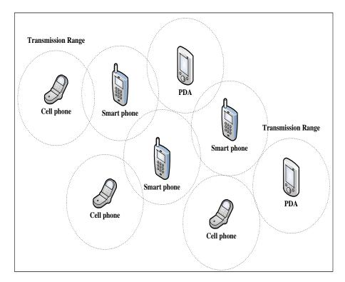
Figure 1-2: Example of a wireless mobile ad-hoc network.
