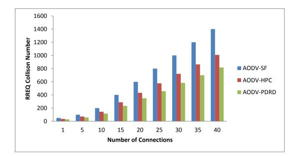
Figure 3-13: RREQ collision number VS. number of connections for a network of 100 nodes in 1000m x 1000m area.
