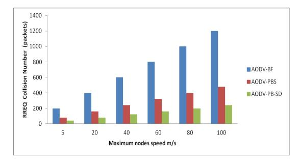
Figure 5-7: Performance of the proposed schemes in terms of RREQ collision number vs. maximum nodes speed.
