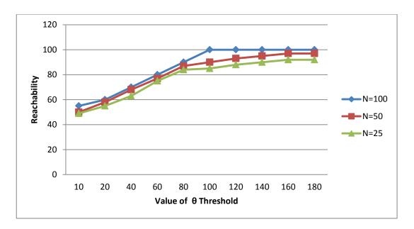
Figure 4-3: RREQ reachability vs. Value of  $\theta$  Threshold over different network densities.
