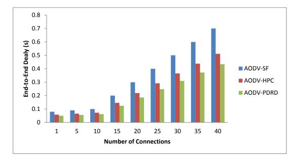
Figure 3-15: end-to-end delay VS. number of connections for a network of 100 nodes in 1000m x 1000m area.
