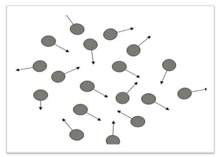
Figure 3-5 : Example of random way point model.
