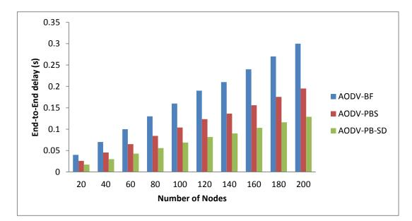
Figure 5-13: Performance of the proposed schemes in terms of end-to-end delay vs. number of nodes.
