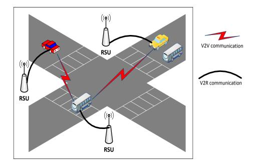
Figure 1-3 : Example of the communication between VANETs components.
