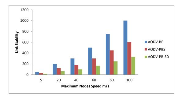
Figure 5-9: Performance of the proposed schemes in terms of Link stability vs. maximum nodes speed m/s.
