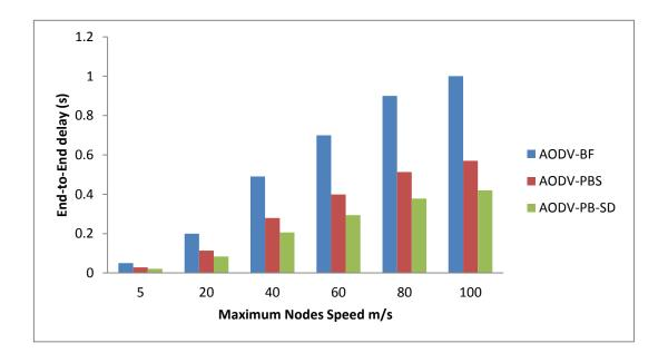
Figure 5-8: Performance of the proposed schemes in terms of end-to-end delay vs. maximum nodes speed m/s.
