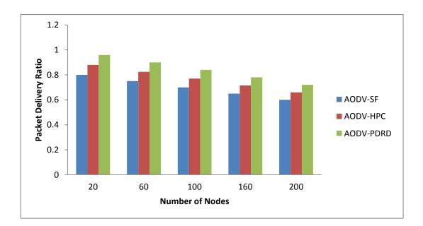
Figure 3-10: shows packet delivery ratio vs. number of nodes for each scheme.
