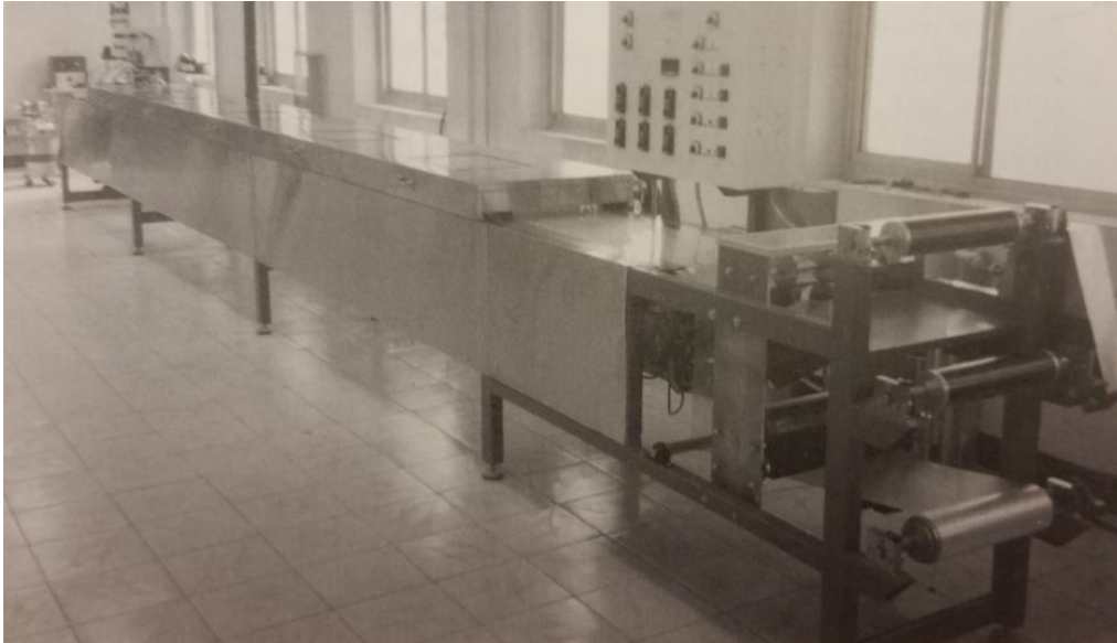
Figure 10 Continuous style tape caster [45]
