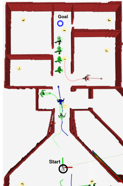
Fig. 6. Start-to-goal query from the Start point (lower side) and the Goal destination (upper side) including a static queue of agents.
