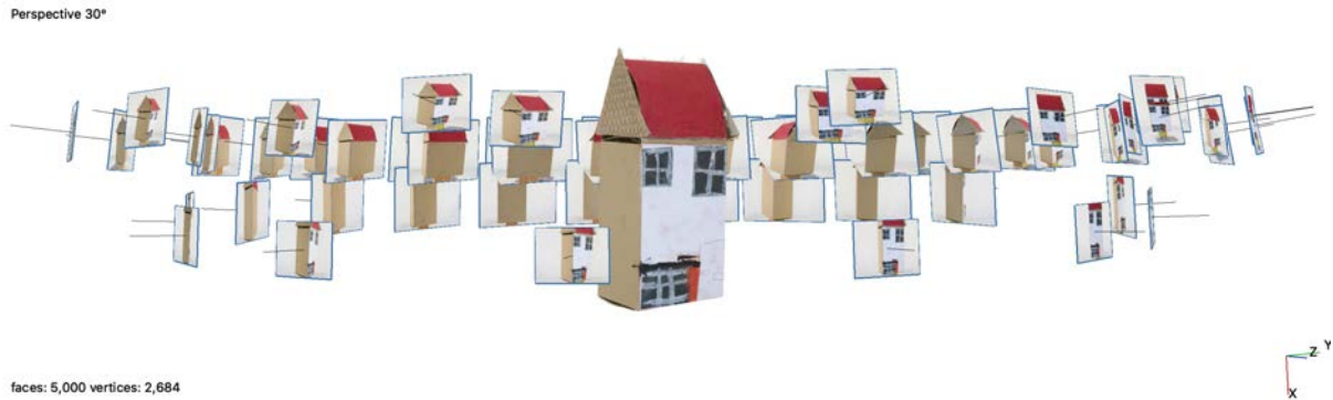
Fig. 6. 3D model of a box-house generated through a photogrammetry automated process
