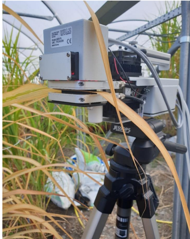
Figure 7.16 Miscanthus leaf being measured by Walz IRGA on 16 th October 2019, 12 days after plants were treated with one of four applications of ethephon
