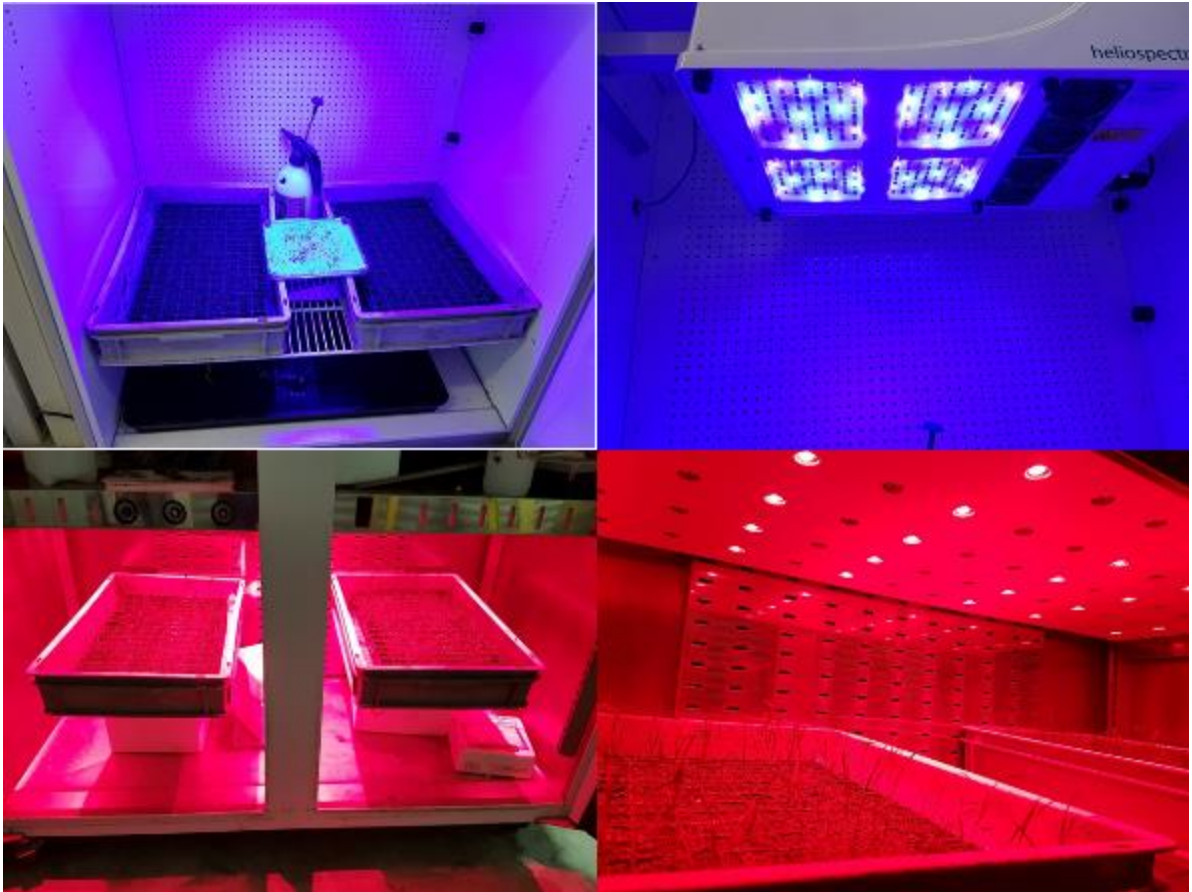
Figure 6.1 Plants in trays in blue light Conviron cabinet, and red light Fitotron cabinet. Plants received no other light source except when cabinet was opened for watering or measuring.
