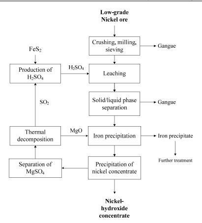
Fig. 1. Proposed flow-sheet for processing of Serbian laterite ores from Rudjinci ore
