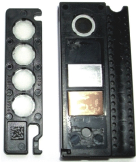
Figure 2. The OSLD components: a slider containing detector elements, and a filtered holder
