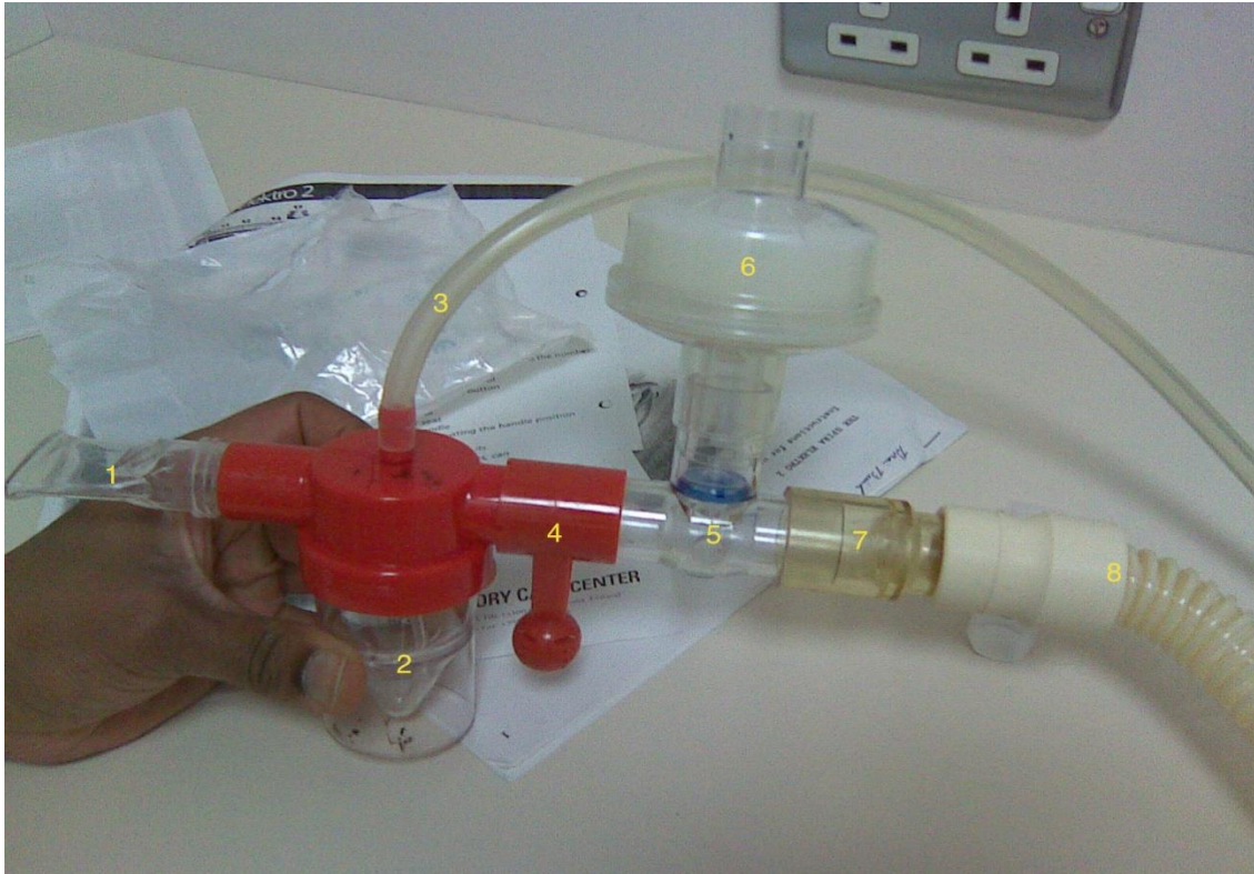
Figure 2.2. Set up of nebuliser equipment. 1 = mouthpiece, 2 = nebuliser chamber, 3 = nebuliser pressure tube, 4 = holder arm, 5 = 'T' piece (exhalation valve), 6 = single-use filter, 7 = tube connector, 8 = participant tube (adapted from L.Barr, monocytes working document 4.0, 2010)
