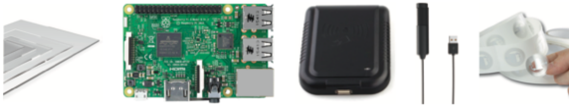
Figure 18: JigsAudio Components (Left to right: Perspex, Raspberry Pi, RFID Reader, USB Microphone and RFID Tags/Stickers)
