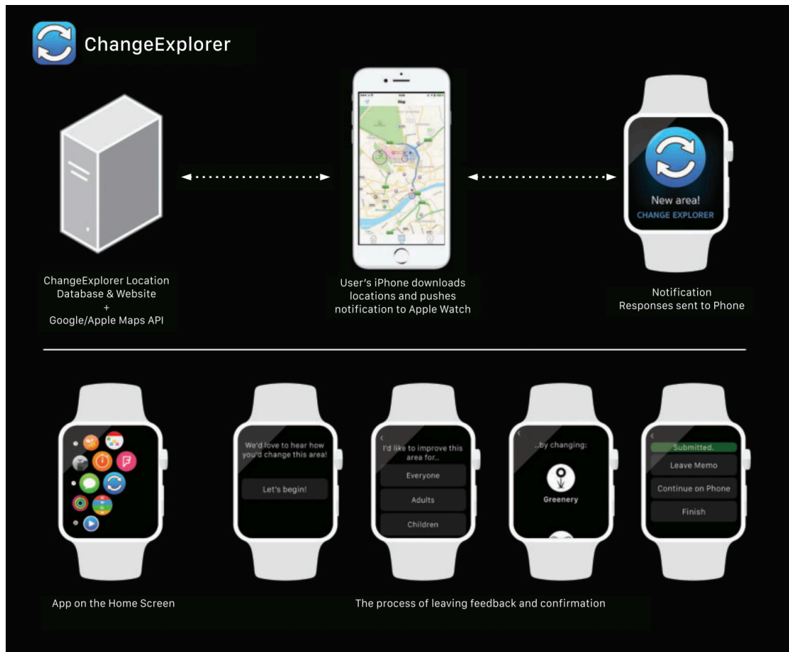
Figure 14: Details of ChangeExplorer’s client server architecture and screen shots of the watch’s interface; screen shots of the notification being received, the app on home screen, and the process of leaving feedback and confirmation
