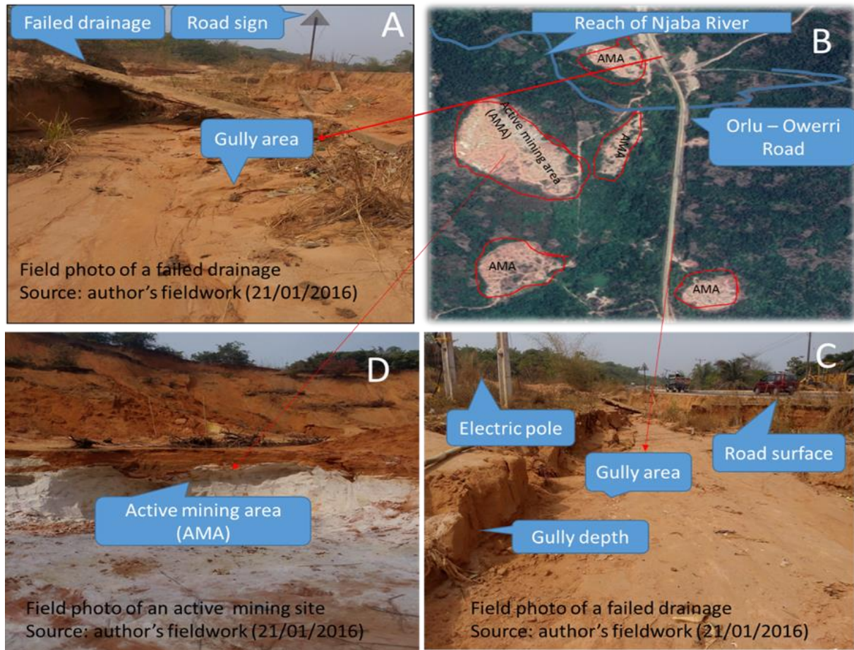
Figure 7-1 Remote sensing locations and field photos of mining sites and infrastructures affected by gullies in Oguta Lake watershed. Source: author's fieldwork and USGS https://earthexplorer.usgs.gov 05 42' 06.8''N 006 00' 36.2''E
