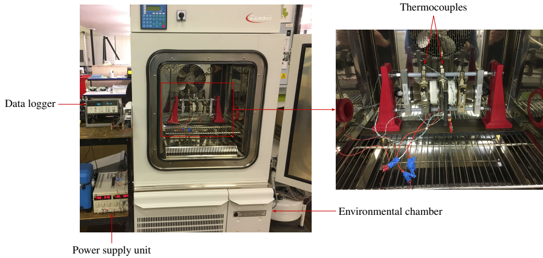
Fig. 6.17. TSEP calibration test setup.
