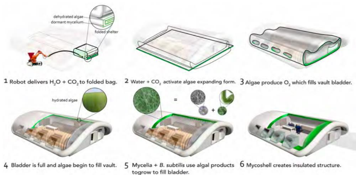
Figure 5.5. Growth of Myco-Architecture on the Martian surface where water, CO 2 , and heat are delivered by robots to promote algal activity which will feed mycelium and Bacillus subtilis to produce inhabitable structures (Rothschild et al. , 2019).
