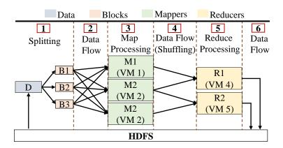
Figure 3.1: An overview model of MapReduce processing and data flow phases
