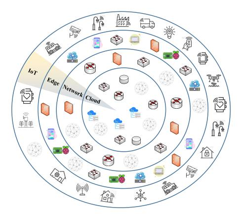
Figure 6.1: 4-tier architecture – the outer layer is composed of IoT devices generating data and transmitting these to Edge devices (second layer). The Innermost layer is comprised of a Cloud datacenter, with a data network connecting these layers
