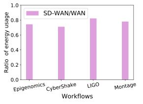
Figure 5.17: Energy consumption in a small-scale SDWAN/WAN - very large size workflows
