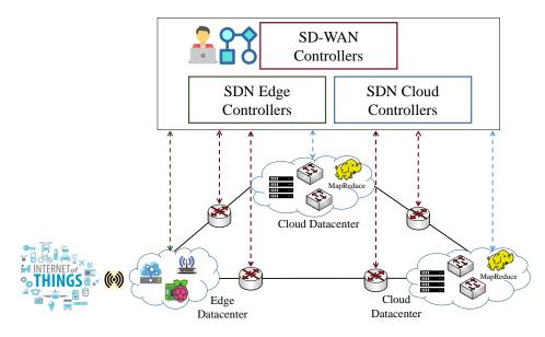
Figure 1.1: An overview of SDN usage and deployment in several environments
