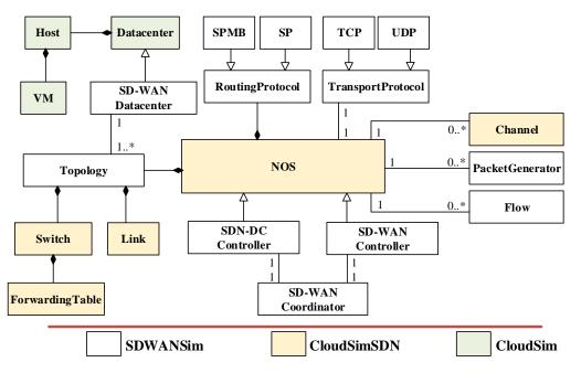
Figure 4.7: System structure of IoTSim-SDWAN
