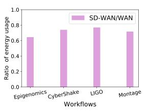
Figure 5.16: Energy consumption in a small-scale SDWAN/WAN - large size workflows
