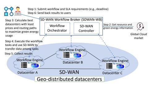
Figure 5.1: High level system model for executing data-driven applications
