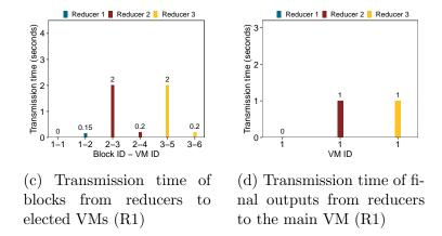
Figure 3.11: Transmission time of MapReduce in a traditional network (R1)
