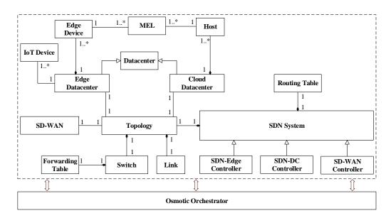
Figure 6.4: IoTSim-Osmosis system components
