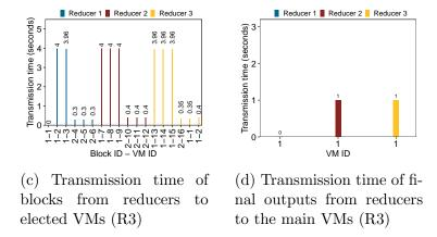
Figure 3.16: Transmission time of MapReduce in SDN load balancing network (R3)
