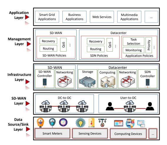
Figure 4.1: Architecture of distributed enterprise ecosystems and SD-WAN
