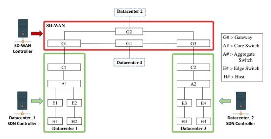
Figure 4.4: Multi-datacenters and SD-WAN topology for experiments.
