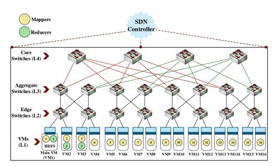
Figure 3.9: Fat-tree topology used in the simulated use-case experiments
