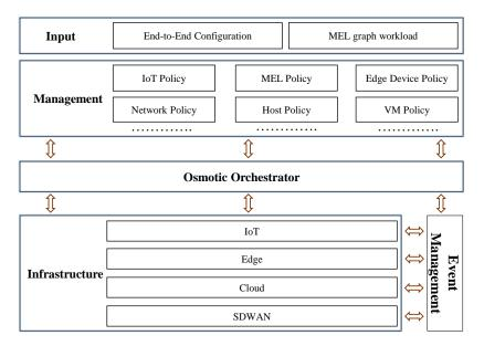
Figure 6.3: Architecture of IoTSim-Osmosis simulator
