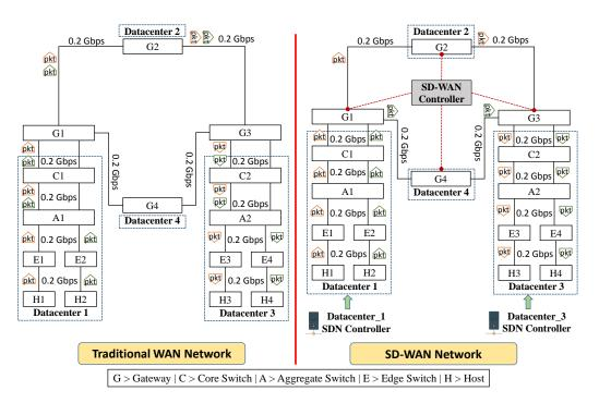
Figure 4.14: Network topology used in IoTSim-SDWAN
