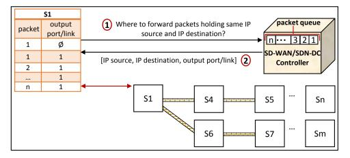
Figure 4.9: An interaction between OpenFlow switches (S#) and SDN for obtaining flow entry
