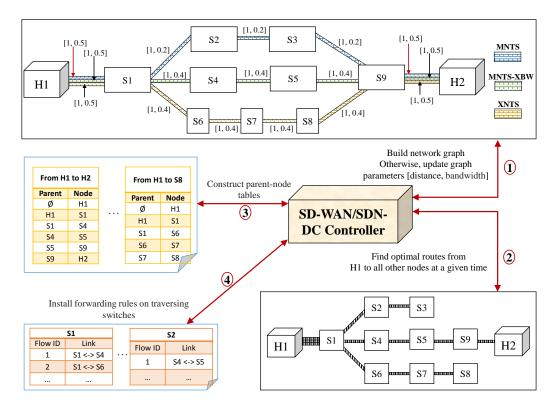
Figure 4.5: Overview of SD-WAN/SDN-DC controller's actions to build forwarding rules. H#: host, S#:switch, MNTS: minimum number of traversing switches, XBW: maximum bandwidth of traversing switches, XNTS: maximum number of traversing switches.
