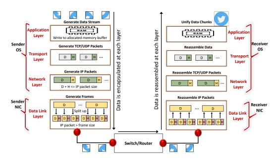
Figure 4.2: Procedure of data transmission based on the TCP/IP model
