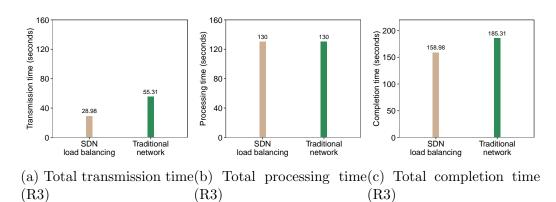
Figure 3.17: Performance comparison of MapReduce between a traditional network and SDN load balancing (R3)
