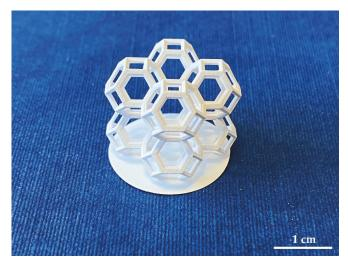
Figure 7. Lattice structure in ATZ printed by the DLP technique.
