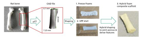
Figure 3. Reverse-engineering workflow from rat bone to a CAD file to the manufactured Freeze Foams and hybrid foams (artificial *corticalis* case).
