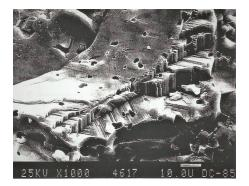
Figure 10. Fractured surface of Mg-PSZ.
