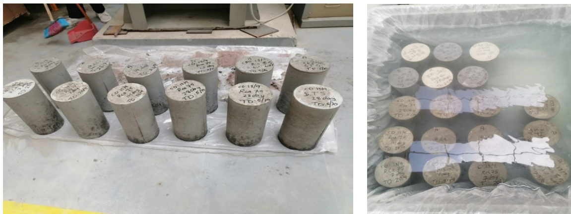
Figure 3. Concrete cylinder demolding and curing.
