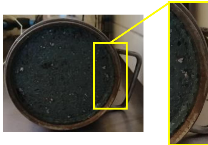
Figure 3. Blue specimen with an excess of bitumen.
