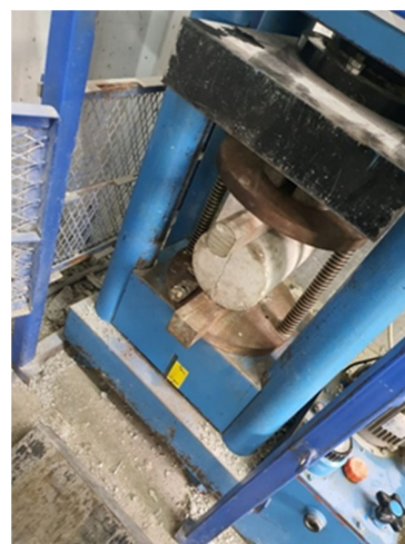
Figure 5. Split tensile strength test.
