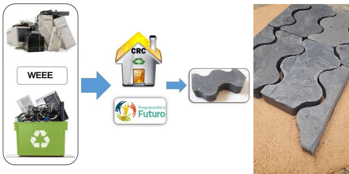
Figure 1. (left) From e-waste to interlocking plastic pavers: the recycling way. Containers to collect e-waste are distributed in strategic points (malls, supermarkets etc.). The Computer Reconditioning Centers (CRC) also collects electronic equipment either in public or private institutions. (right) On a sand bed, the pavers form a pavement with space for accommodation and drainage.
