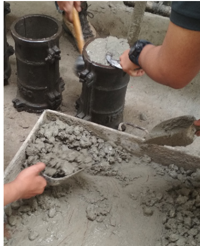
Figure 3. Preparation of concrete cylinder specimen.
