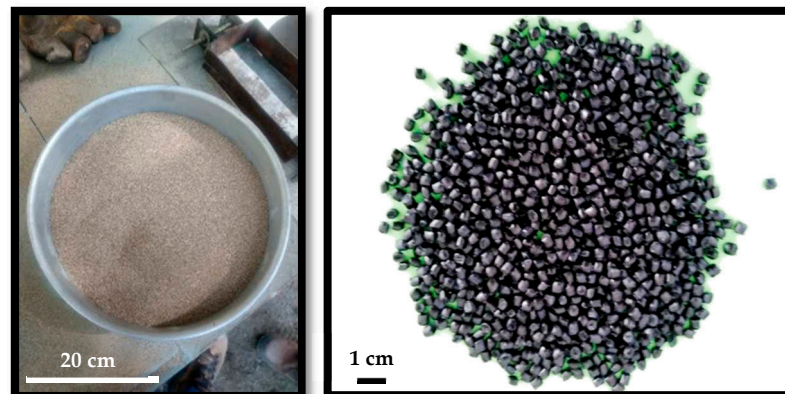
Figure 1. Sand and plastic pellets used in the manufacturing of plastic sand cobbles.
