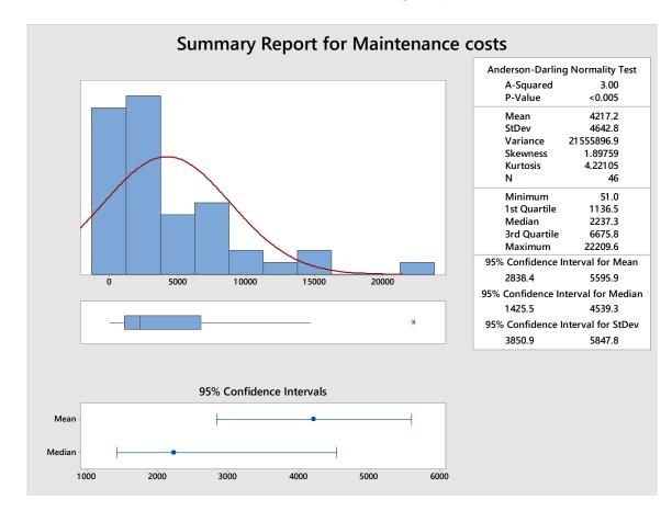
Figure 3. Normality test for maintenance costs.
