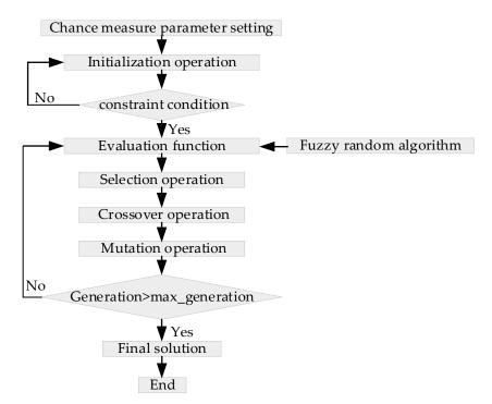
Figure 7. Hybrid intelligent algorithm flow chart.
