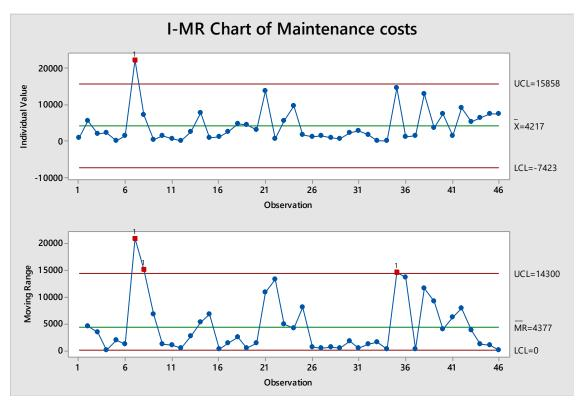
Figure 4. Stability of the maintenance costs process.
