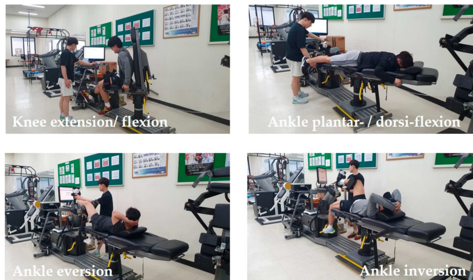
Figure 4. Isokinetic moments measures' samples. The knee joint for knee extension and flexion was positioned at 90°. All participants were concentrically tested at 60°/s and 180°/s. The test angles for ankle plantarflexion and dorsiflexion comprised of movement from 50° (plantarflexion) to 20° (dorsiflexion), where all participants were concentrically tested at 30°/s and 120°/s. The test angles for ankle inversion/eversion comprised of movement from 55° (inversion) to 40° (eversion), where all participants were concentrically tested at 60°/s and 90°/s.
