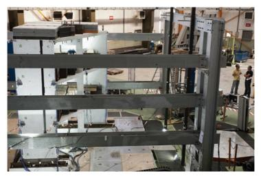
**Figure 10.17** The SMART2011 instrumented mock-up (used in support of a joint research program between CEA and EDF) is representative of a 1/4-scale "nuclear" building. Weighing around 47 tonnes (including 36 tonnes of additional weights), SMART2011 was instrumented with more than 200 measurement channels (acceleration, displacement, deformation) and was subjected to a series of seven earthquakes of increasing magnitude. © P. Stroppa/CEA.
