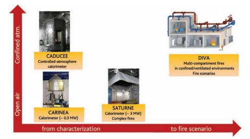
**Figure 7.2-a** Positioning of the different types of fire characterization test in relation to the test facilities. @ Laurence Rigollet/IRSN.
