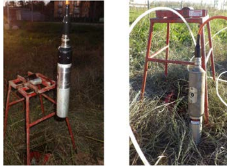
Figure 1.21 Hydrophone with an amplification system and 3C geophone with an anchoring system (Solgé).
