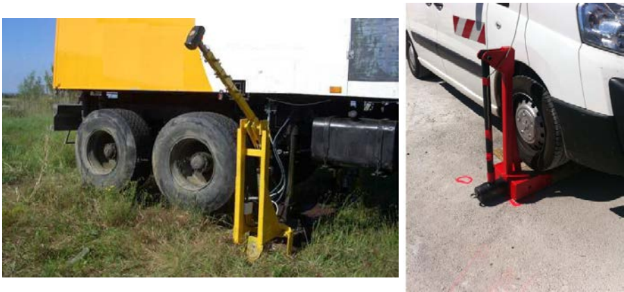
Figure 1.4 Illustration of an S source used in downhole testing which complies with the ASTM standard (lgeoTest source on the left, IMG source on the right).
