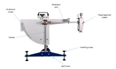
Figure 25. A typical commercial British Pendulum.
