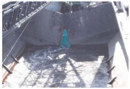
Figure 5 - Opening which enable the water to fill the housing for the clods.
