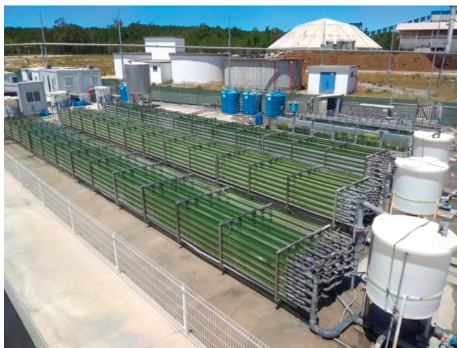
Figure 1. Pilot-scale tubular photobioreactors (PBRs) used in the trials with 2.6 \text{m}^3 of working volume (Almmicroalgae, Pataias, Portugal).
