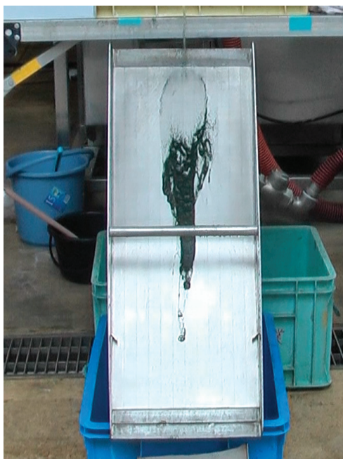
Figure 4. Harvesting of B. braunii cultured in the brackish medium (BM) using an inclined solid–liquid separator with a wedge-wire screen (150 \mu\text{m} slit size).
