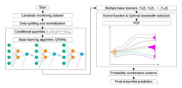
**Figure 2.** The overall flowchart of ensemble prediction based on the quantile regression neural networks and kernel density estimation (QRNNs-KDE) approach.
