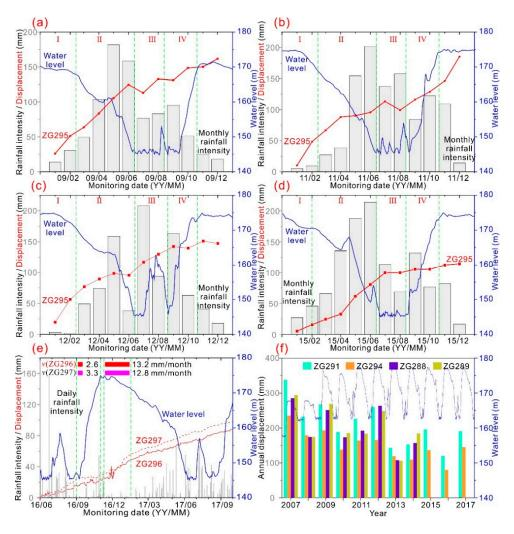
**Figure 6.** (**a**–**d**) Cumulative displacement at monitoring point ZG295, monthly rainfall intensity, and reservoir water level spanning the period of 2009, 2011, 2012, and 2015. (**e**) Cumulative displacement at monitoring points ZG296 and ZG297, daily rainfall intensity, and reservoir water level spanning the period of June 2016 to October 2017. (**f**) Annual displacement at monitoring point ZG291, ZG294, ZG288, and ZG289, and reservoir water level spanning the period of 2007 to 2017.
