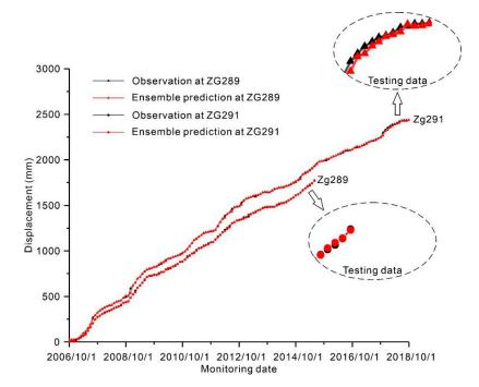
**Figure 9.** Comparisons of the final ensemble predictions and observations for the Fanjiaping landslide at ZG289 and ZG291.
