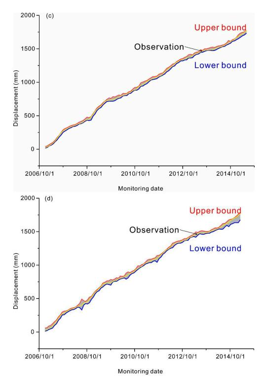
**Figure 10.** Comparisons of the observations and the constructed PIs at a 90% confidence level for the Fanjiaping landslide at ZG289 and ZG291 using QRNNs-KDE and bootstrap-ELM-ANN. (**a**) 90% PIs at ZG291 using QRNNs-KDE; (**b**) 90% PIs at ZG291 using bootstrap-ELM-ANN; (**c**) 90% PIs at ZG289 using QRNNs-KDE, (**d**) 90% PIs at ZG289 using bootstrap-ELM-ANN.
