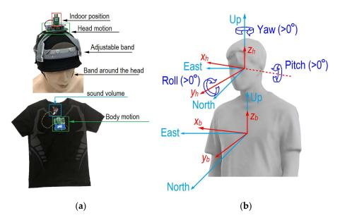
**Figure 2.** Device design and motions of head and body. (a) Device for indoor positioning, and head and body motion detection; (b) current and base vectors for head and body.
