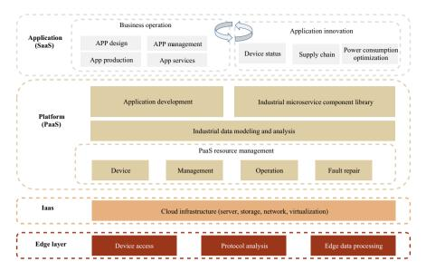
Fig. 11.1 Architecture of the industrial internet platform. *Source* Industrial internet platform whitepaper released by Alliance of Industrial Internet in 2017, CICC Research. *Note* SaaS refers to software as a service, PaaS refers to platform as a service, IaaS refers to infrastructure as a service
